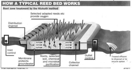
9.2 Industrial wastewater recycling/treatment with flow through system.
