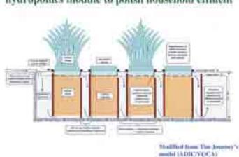
Schematic drawing of proposed vetiver hydroponics module to polish household effluent
