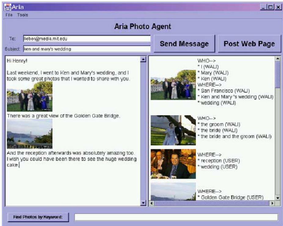
Fig. 1. A screenshot of ARIA which combines an email panel (left) with a photo database (right) that dynamically reorders itself in real-time, as the user types
