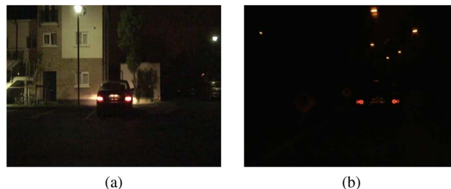
Fig. 1. Example of (a) video frame captured with the automatic exposure control enabled and (b) video frame captured using a lower static exposure [ EV_{100} = 10 ]. Note how the rear lights in (a) saturate, resulting in the lights appearing white, whereas, in (b), the color of the red lights is preserved. However, in (b), much of the lower intensity background detail from the scene is not present, due to the lower exposure.
