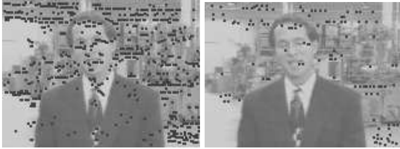
Figure 4: Left: All instances of horizontal edges. Right: All instances of a local feature dedicated to faces.
