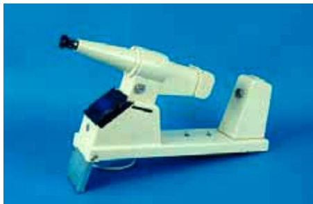
Figure 5: Photograph of the Nagel anomaloscope (Model I, Schmidt and Haensch, Germany) and illustration of the Nagel anomaloscope split field. The percentage mixture of red to green in the top half and the luminance of the yellow bottom field can be changed until a match of the two fields can be perceived.
