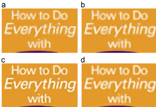
Fig. 11. Super-resolved images: Words. (a) Chang's algorithm. (b) Tang's algorithm. (c) Yang's algorithm. (d) Algorithm 1.
