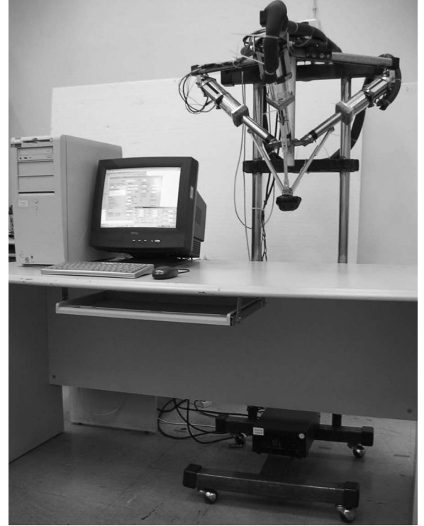
Fig. 7. Photograph of a 3-PUU medical parallel robot prototype.
