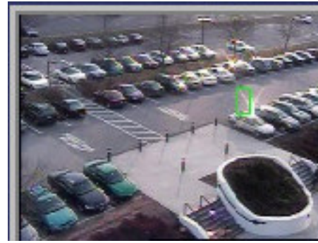
Figure 3. Example of false positive due to specular reflection which is removed by track post processing.
