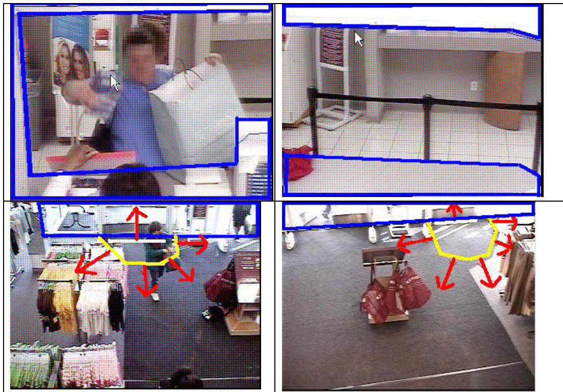
Figure 16: Views from four of the six cameras — two at the customer service desk (top) and two of the four doors (bottom). The “region of uninterested” is shown in blue for all frames and the entrance tripwires (enter in yellow, leave in white) are drawn on the views.
