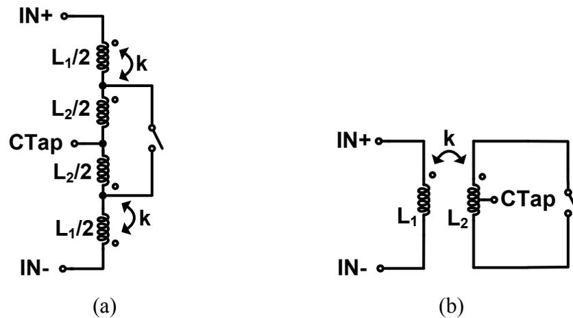
Fig. 3.6: Inductance tuning methods (a) switched inductor (b) switched mutual coupling.
