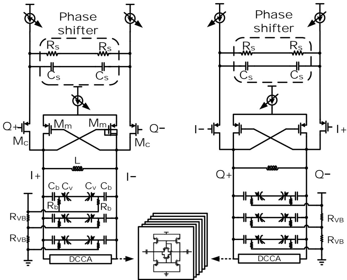
Fig. 4.4: QVCO with the proposed phase shifter.
