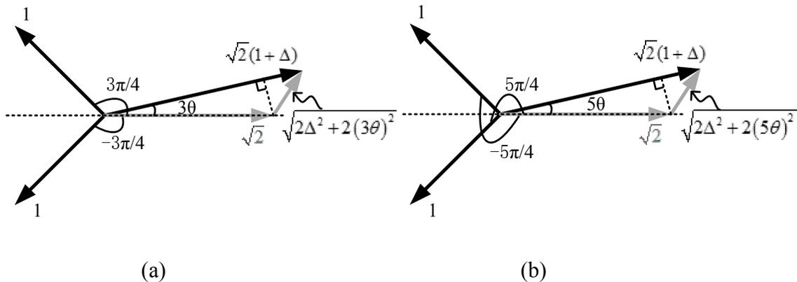
Fig. 4.9: Residual harmonics due to phase and gain mismatches: (a) third-order harmonic, and (b) fifth-order harmonic.
