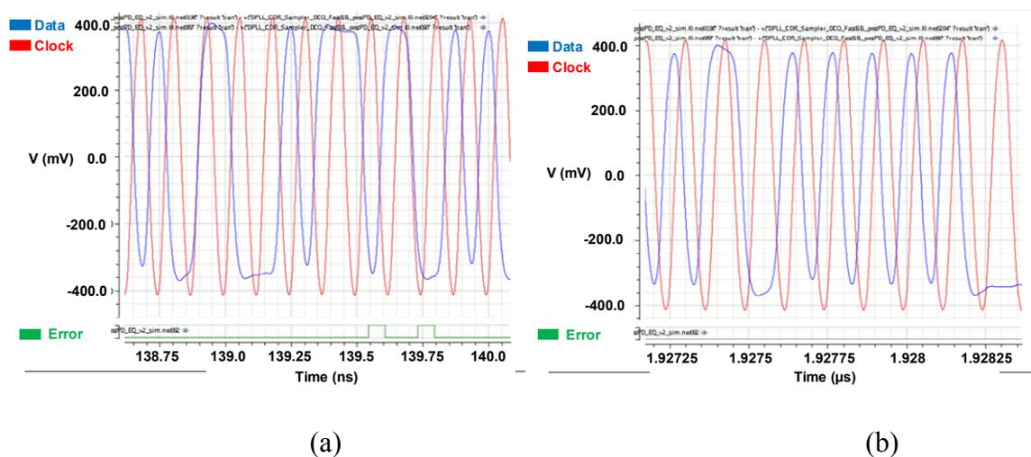
Fig. 3.46: CDR 1:16 deserializer inputs (a) CDR is unlocked (b) CDR is locked.
