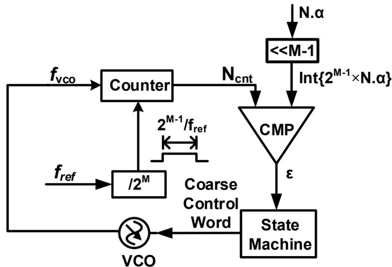
Fig. 2.13: Counter-based AFC.
