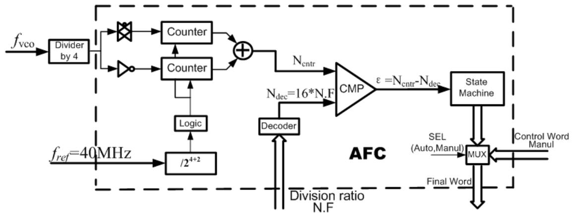
Fig. 4.11: AFC for coarse frequency tuning.
