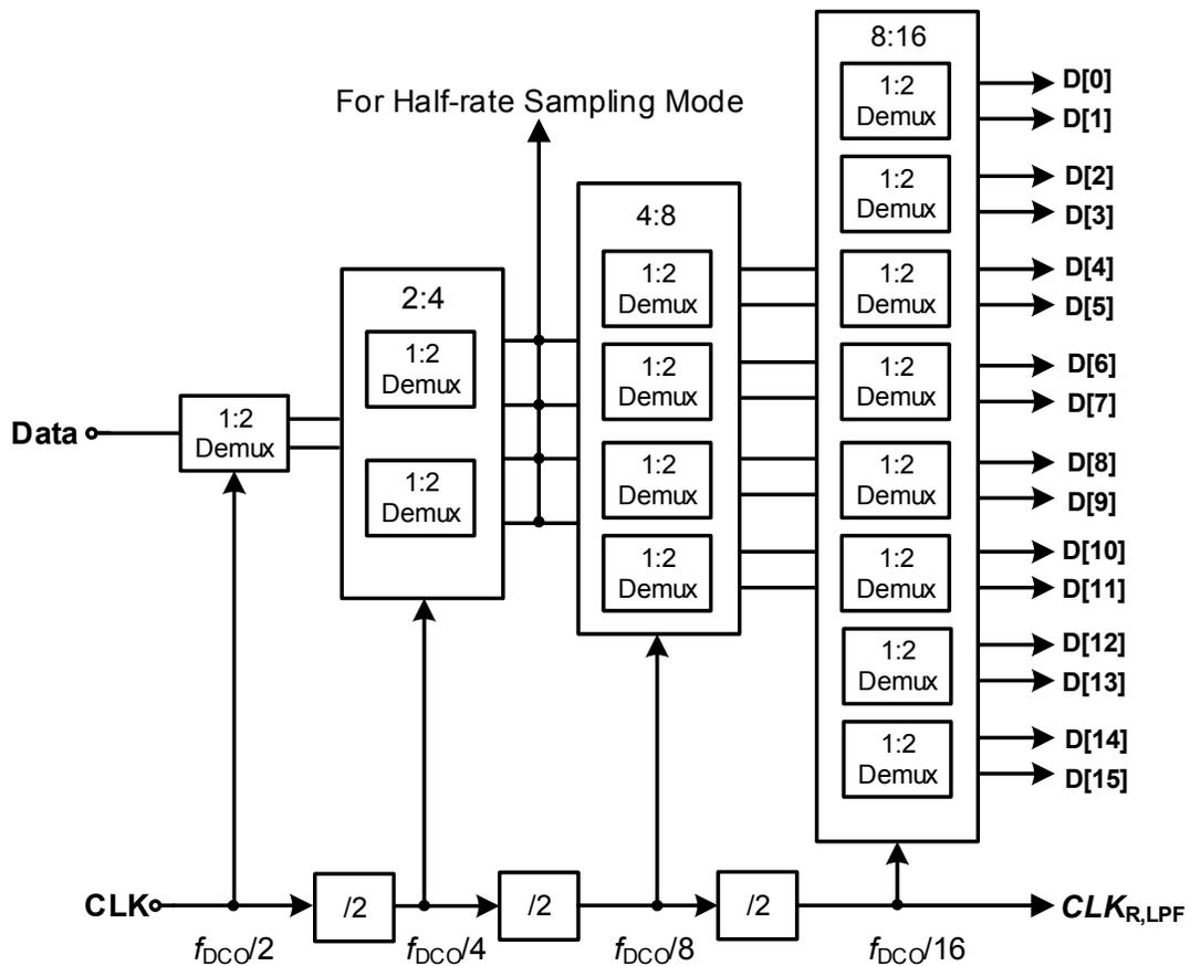
Fig. 3.4: Block diagram of the 1-to-16 de-serializer.
