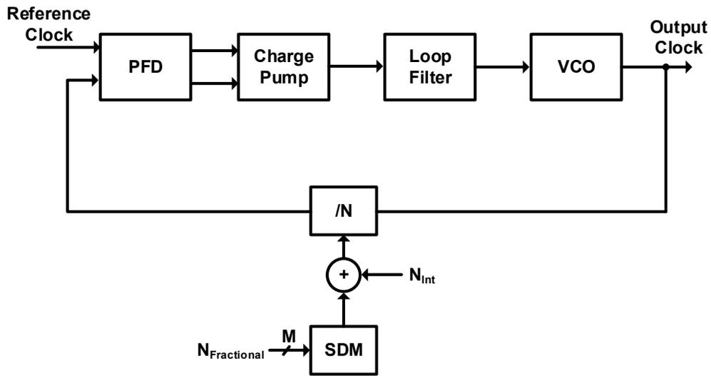
Fig. 2.8: Block diagram of a fractional-N frequency synthesizer.
