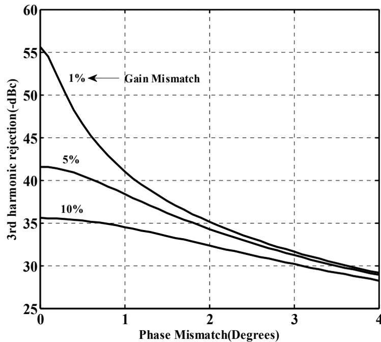
Fig. 4.10: Third-order harmonic rejection with respect to gain and phase mismatches.
