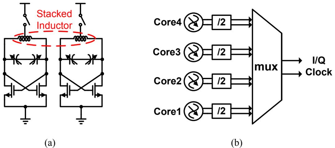
Fig. 3.5: Existing wideband DCO architecture (a) DCO with stacked inductors (b) DCO with multiple cores.
