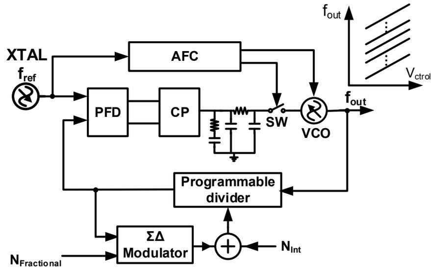
Fig. 2.11: Block diagram of a fractional-N PLL with an AFC loop.
