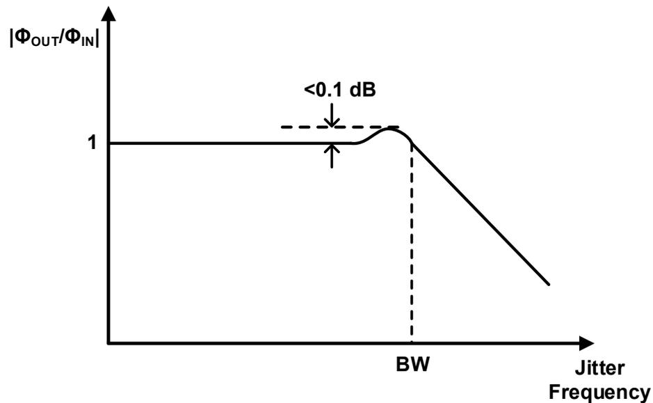
Fig. 2.5: Jitter transfer of a CDR.
