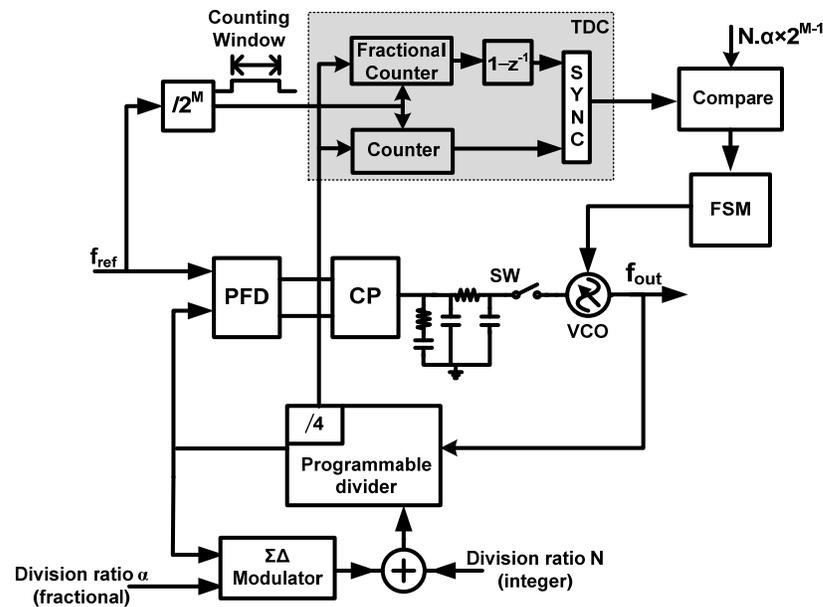
Fig. 5.7: Fractional-N PLL with the TDC-based AFC.
