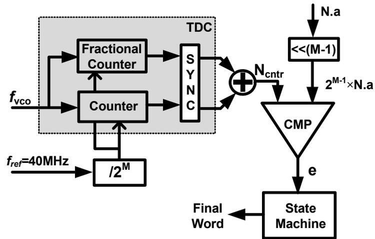
Fig. 5.5: Proposed TDC-based AFC.
