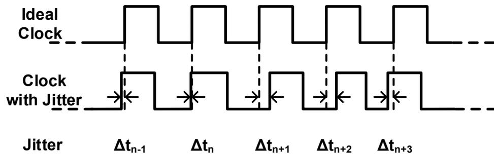
Fig. 2.4: Jitter on a clock signal.
