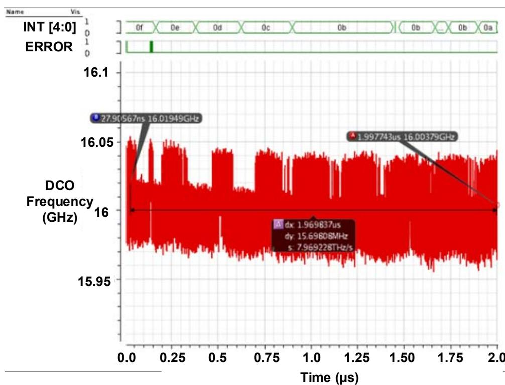
Fig. 3.45: CDR transient simulation result.
