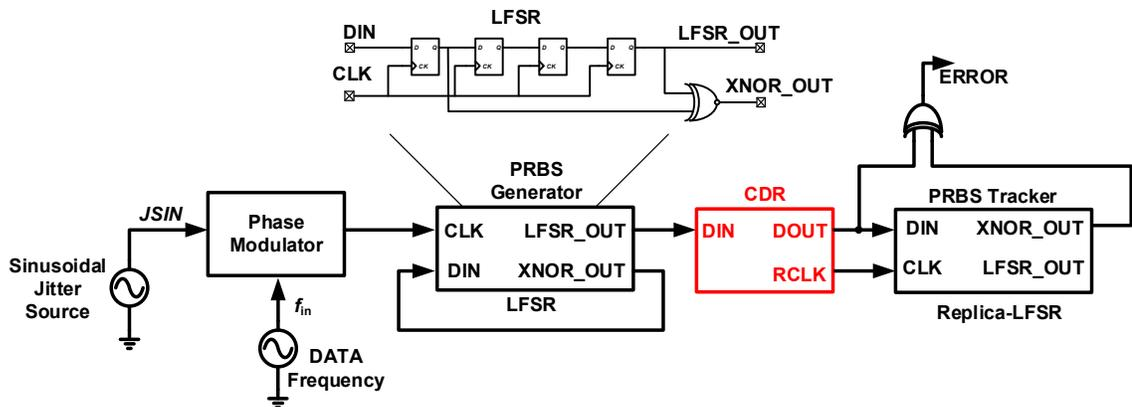
Fig. 3.43: CDR BER simulation setup.
