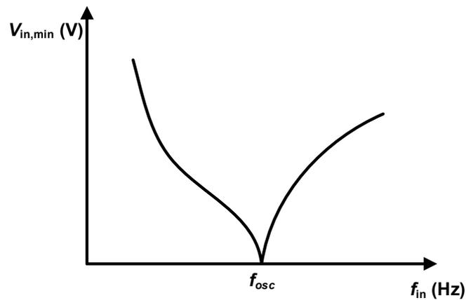
Fig. 3.22: Sensitivity curve for a CML frequency divider.
