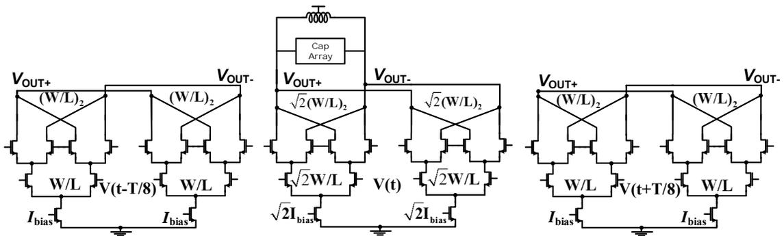
Fig. 4.8: Harmonic rejection SSBmixer.
