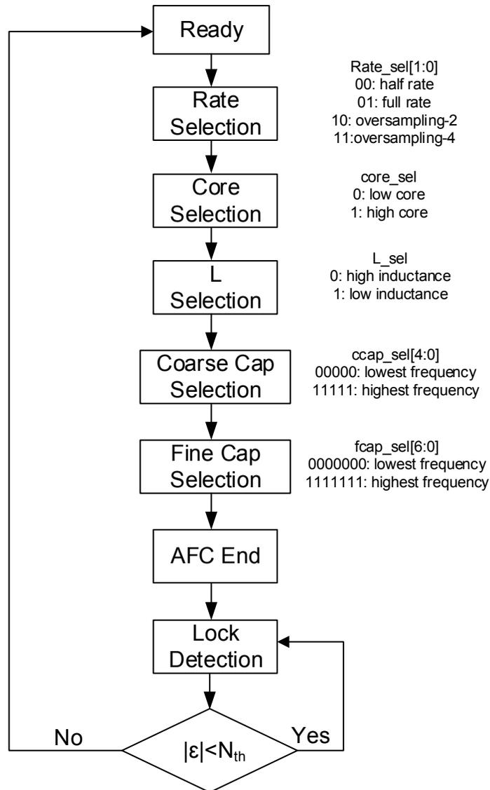
Fig. 3.16: FLL operation procedure.
