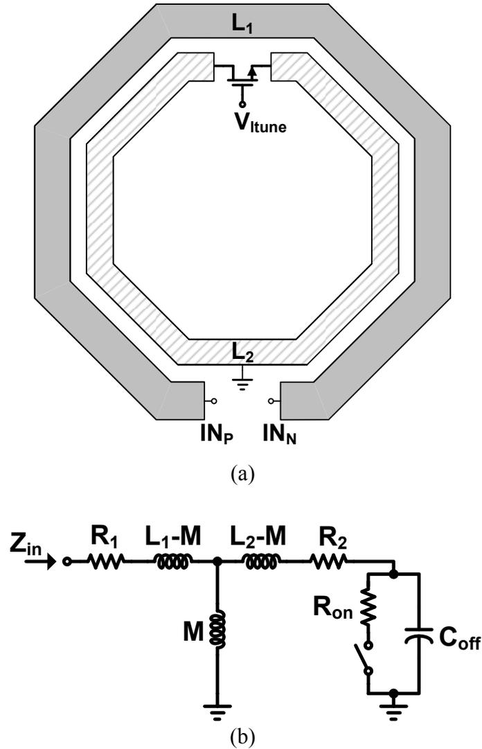
Fig. 3.7: (a) Switched mutual-coupling inductor and (b) its equivalent model.
