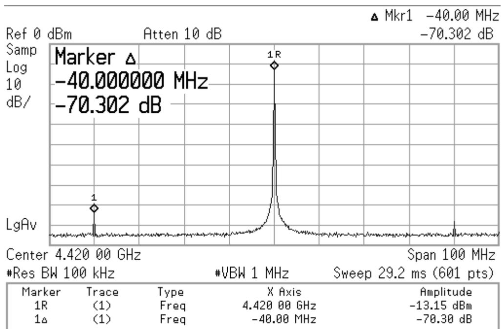
Fig. 4.19: Measured reference spurs.
