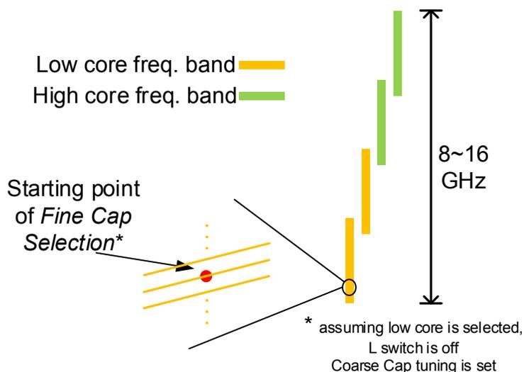
Fig. 3.21: DCO setting at the beginning of *Fine Cap Selection*.
