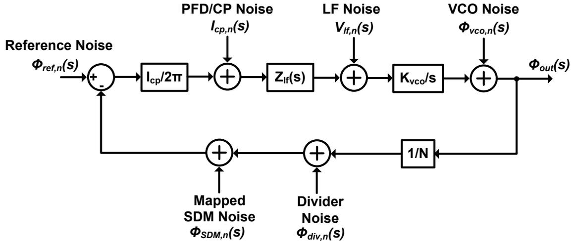
Fig. 2.10: Linear phase noise model of the fractional-N frequency synthesizer.
