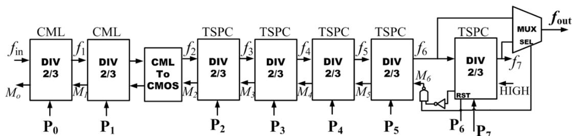
Fig. 4.12: Modular programmable divider.
