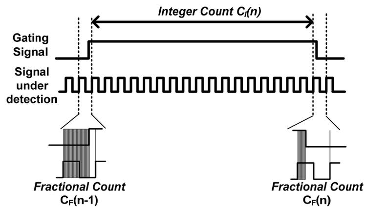
Fig. 5.4: Fractional-counter-assisted frequency detection.
