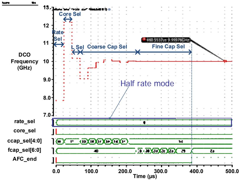
Fig. 3.31: FLL process of 10 Gbps K28.7 data pattern.
