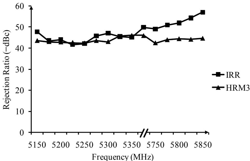
Fig. 4.22: Third-order harmonic rejection and image rejection of the HR-SSBmixer.
