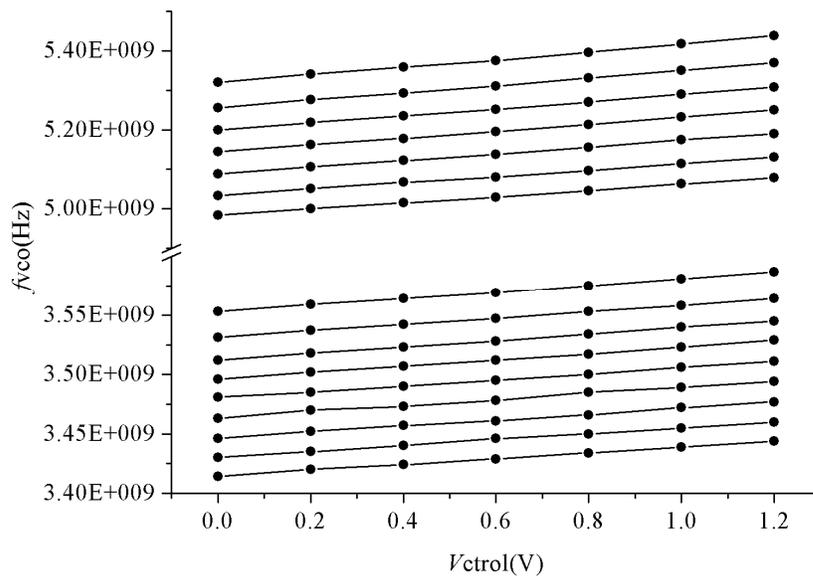
Fig. 4.15: Measured tuning curves of the QVCO.
