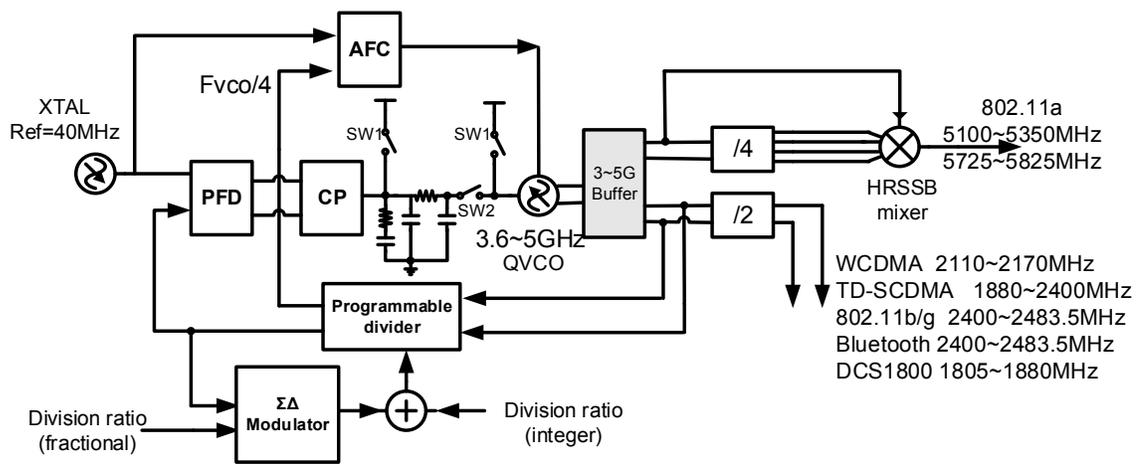
Fig. 4.1: Block diagram of the proposed multi-standard frequency synthesizer.
