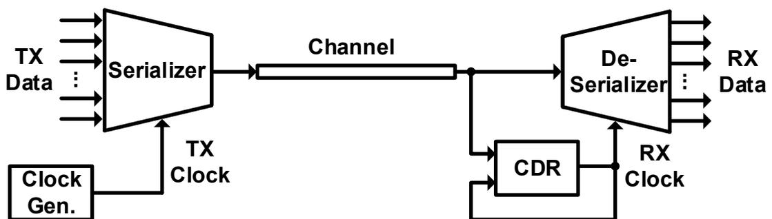
Fig. 1.1: Block diagram of a high speed wireline communication system.
