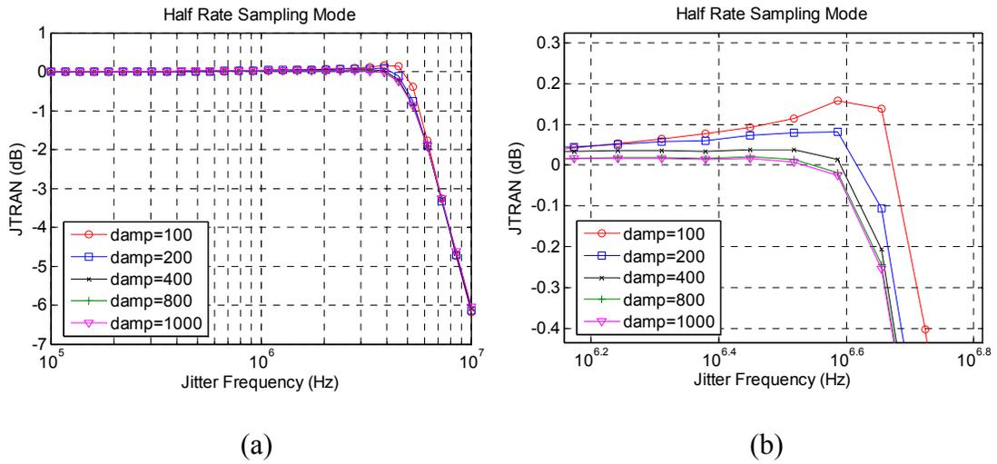
Fig. 3.35: (a) JTRAN and (b) jitter peaking of CDR in the half-rate sampling mode.
