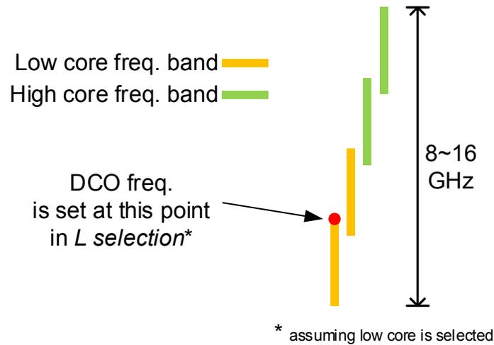
Fig. 3.19: DCO setting during *L Selection*.
