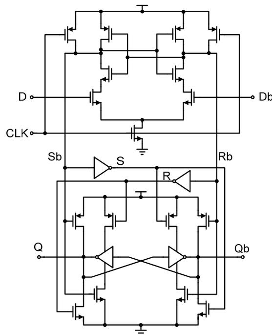
Fig. 5.9: Sense amplifier-based differential D flip-flop.
