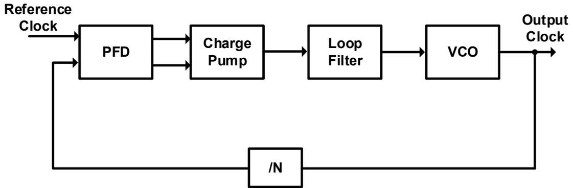
Fig. 2.7: Block diagram of a PLL-based frequency synthesizer.
