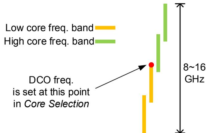
Fig. 3.18: DCO setting during *Core Selection*.
