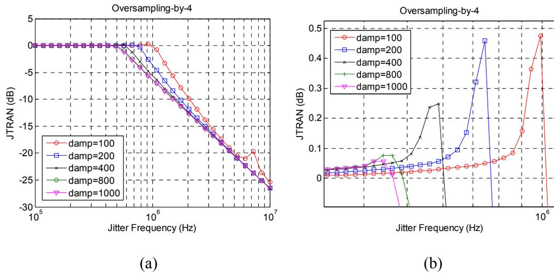
Fig. 3.38: (a) JTRAN and (b) jitter peaking of CDR in the oversampling-by-4 mode.
