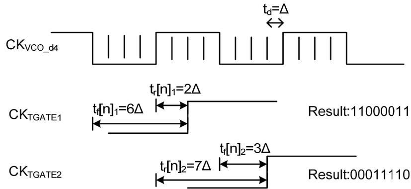
Fig. 5.10: Fractional phase evaluation.
