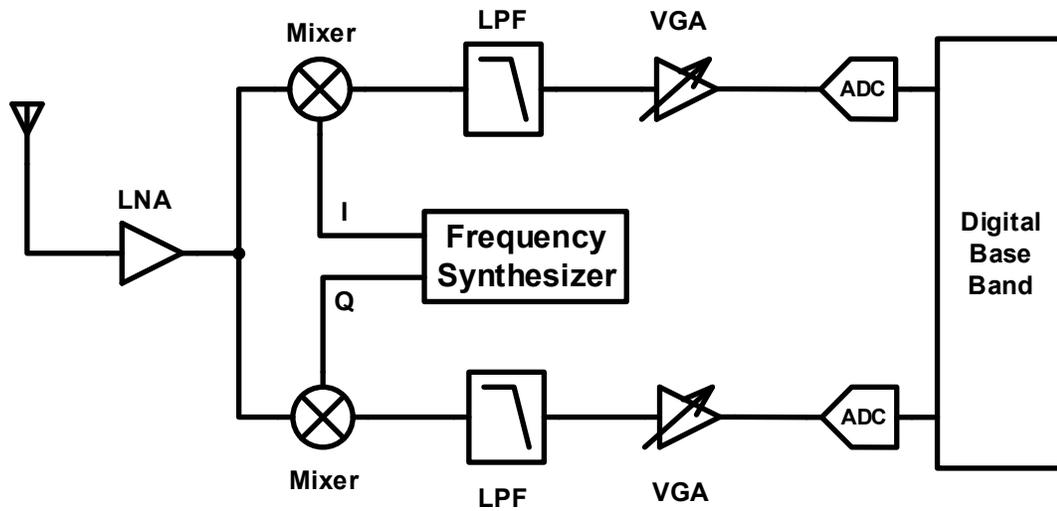
Fig. 1.2: Block diagram of a direct conversion receiver.
