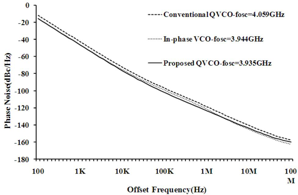
Fig. 4.6: Comparison of the phase noise simulation results.
