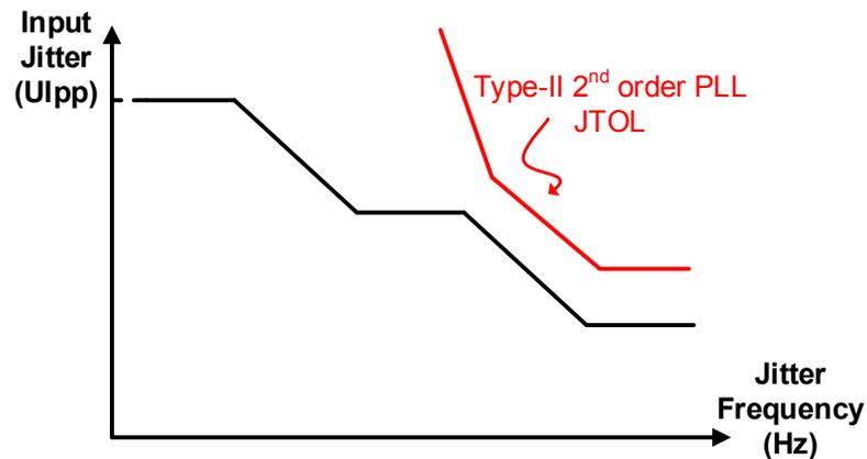
Fig. 2.6: JTOL of a Type-II 2nd-order PLL-based CDR and a typical JTOL mask.
