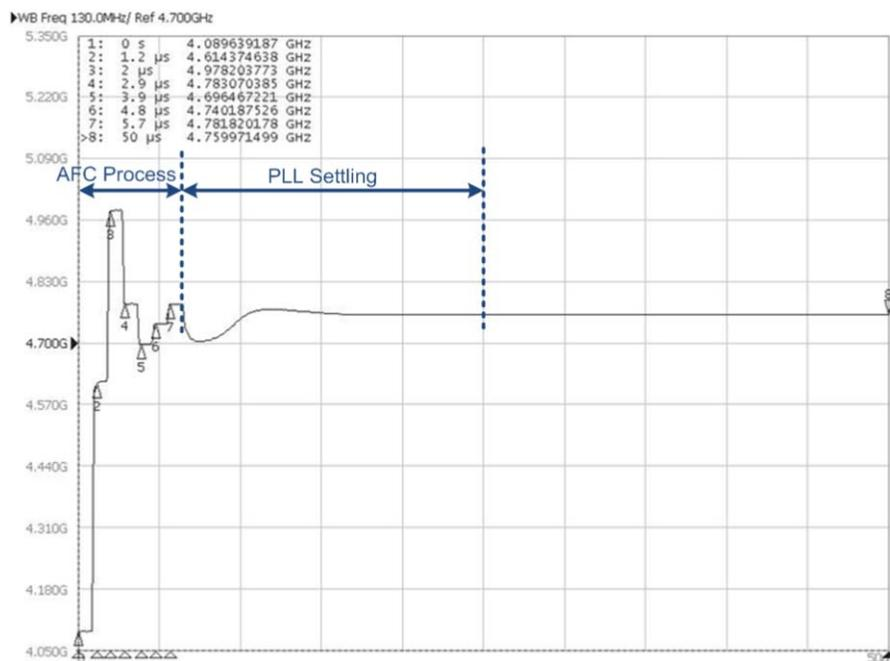
Fig. 4.17: Measured PLL settling time.
