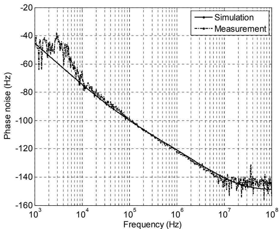
Fig. 4.16: Comparison between simulated and measured QVCO phase noise at 4.09 GHz.
