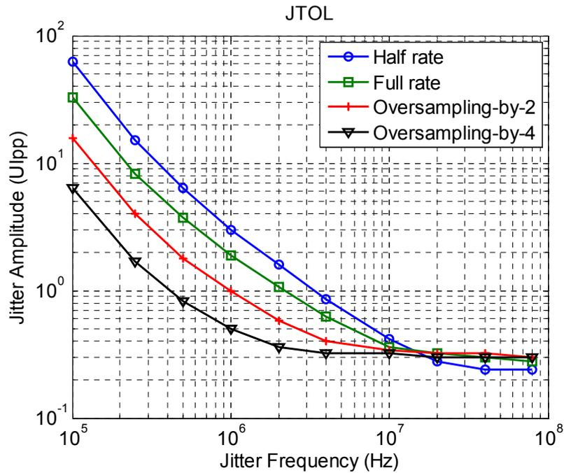
Fig. 3.39: Jitter tolerance simulation results.
