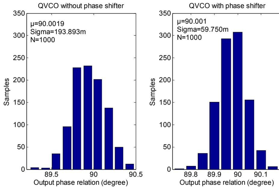
Fig. 4.7: Comparison of the output phase accuracy.
