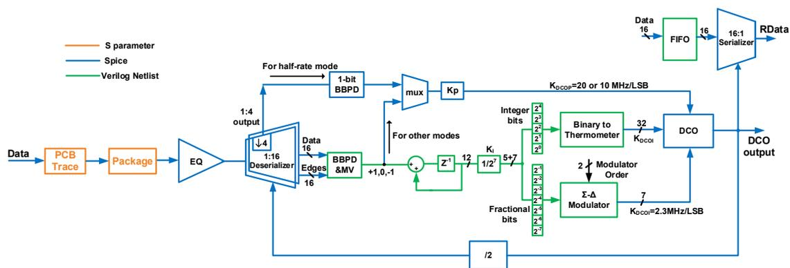
Fig. 3.44: CDR simulation setup.
