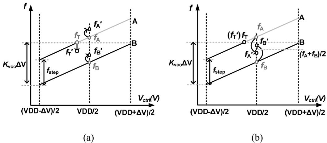
Fig. 5.3: Two worst-case scenarios causing incorrect AFC operation.
