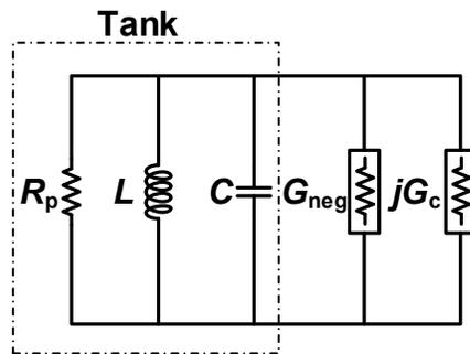
Fig. 4.2: One port model of the QVCO.
