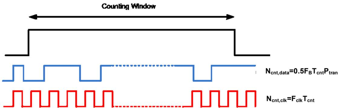
Fig. 3.14: Counting the number of rising edge for data and clock.
