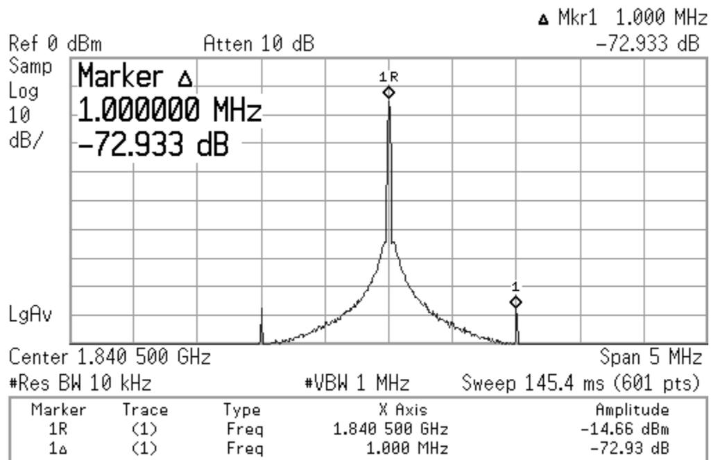
Fig. 4.20: Measured fractional spurs.
