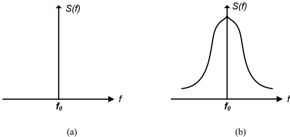
Fig. 2.9: Spectrum of (a) ideal clock (b) realistic clock.
