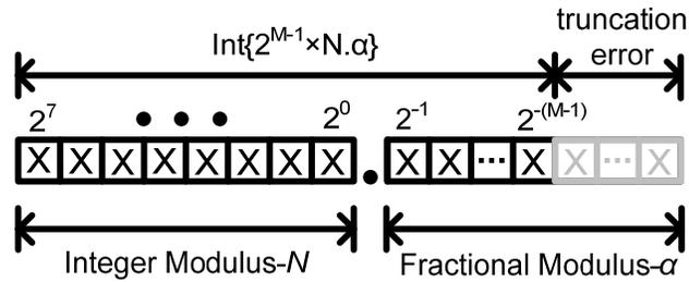
Fig. 5.2: Truncation of the division ratio in the counter-based AFC.
