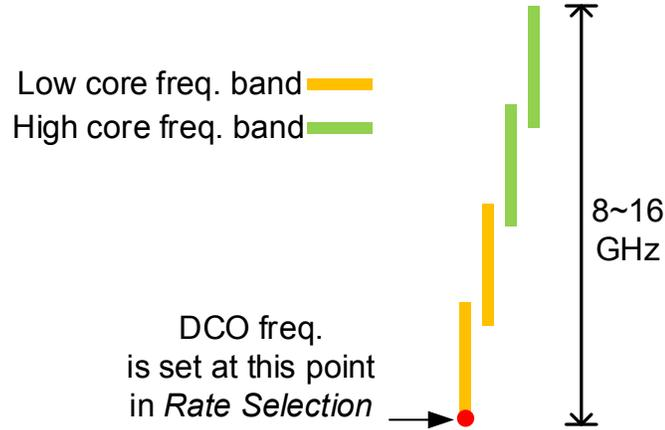
Fig. 3.17: DCO setting during *Rate Selection*.
