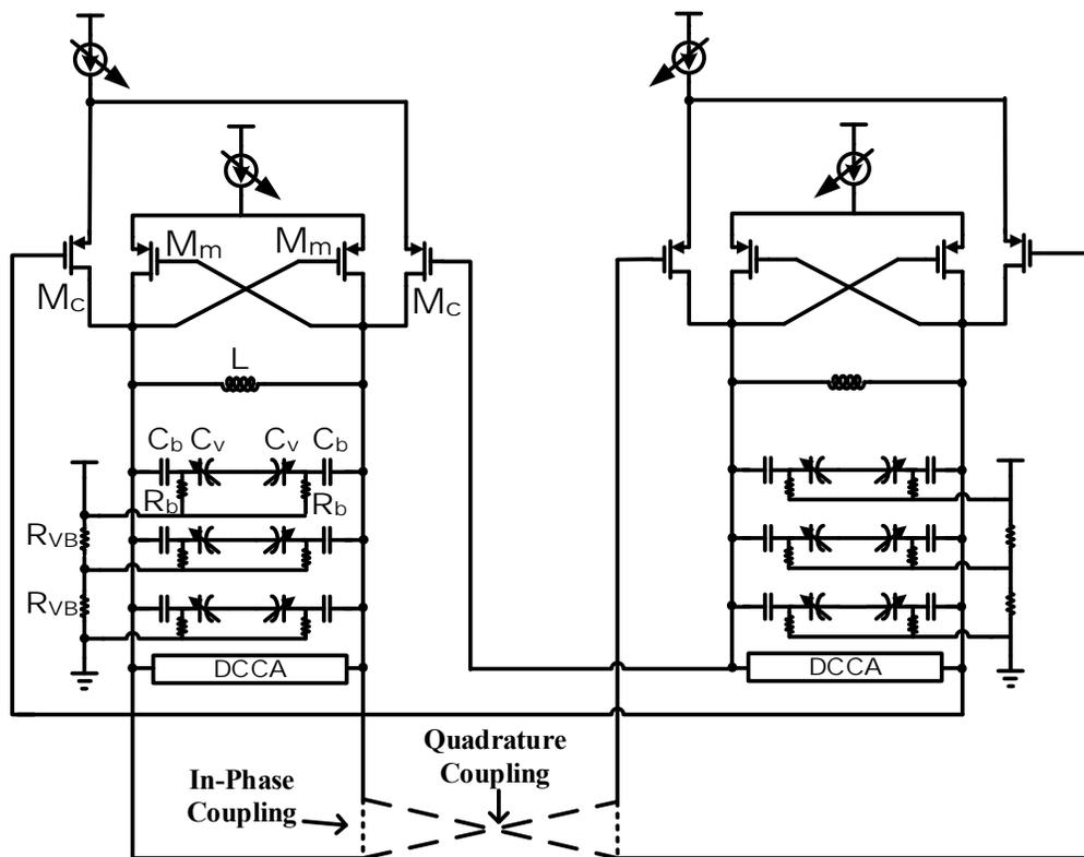
Fig. 4.5: Two oscillators coupled to operate in quadrature and in phase.
