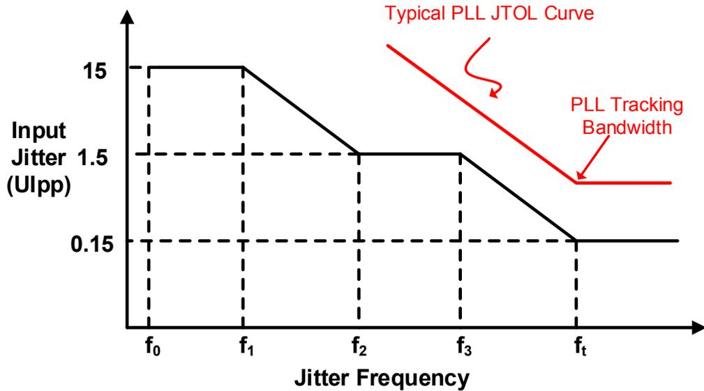
Fig. 3.3: Jitter tolerance mask.
