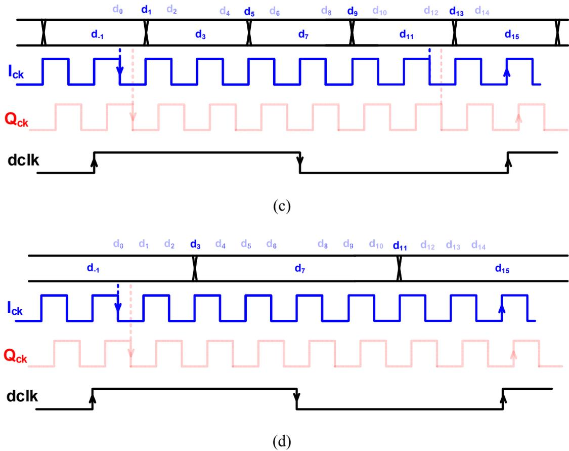
Fig. 3.2: Sampling modes of the CDR (a) Half-rate sampling (b) Full-rate sampling (c) Oversampling-by-2 (d) Oversampling-by-4.
