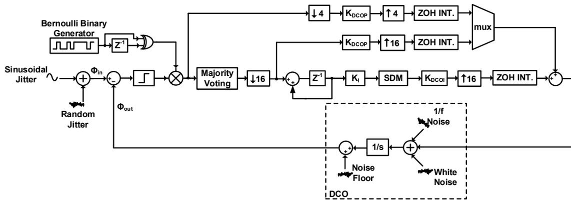
Fig. 3.32: CDR phase domain Simulink model.
