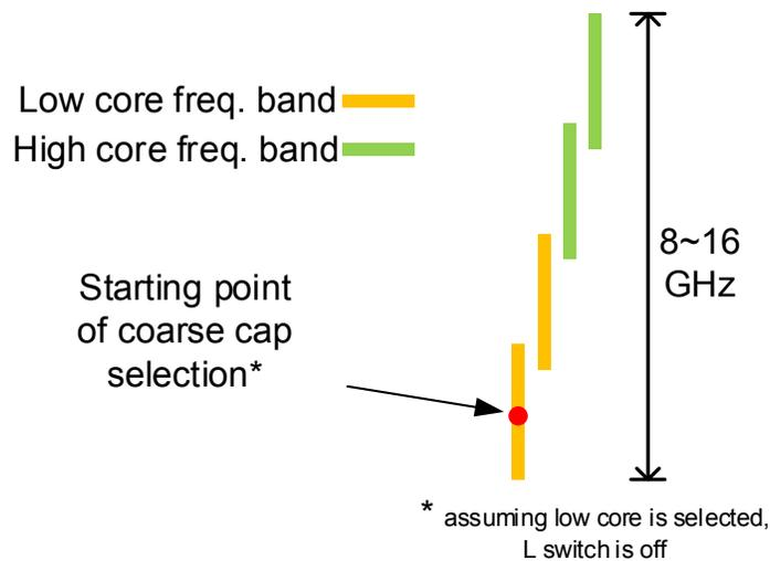
Fig. 3.20: DCO setting at the beginning of *Coarse Cap Selection*.
