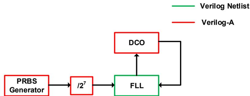
Fig. 3.26. FLL simulation setup.
