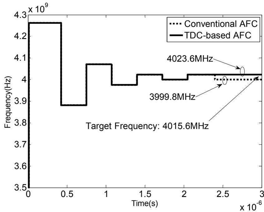
Fig. 5.13: Effect of initial phase uncertainty on the AFC operation.
