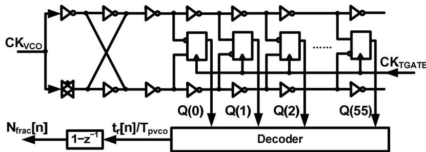
Fig. 5.6: Fractional counter implementation in the TDC-based AFC.
