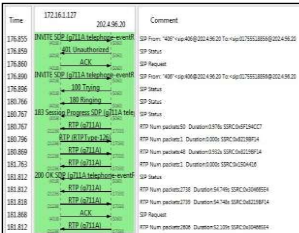
Figure 7. Call flow diagram
