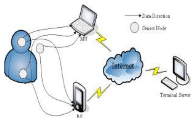
Figure 1. The basic framework of wireless body area network
