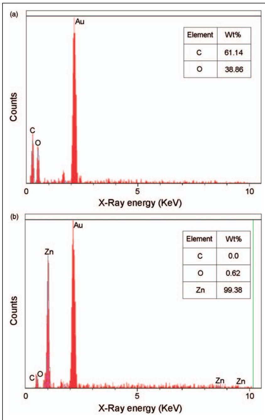
Figure 2. Energy-dispersive X-ray spectroscopy spectra of the control (a) and the ZnO-coated (b) fabrics.
