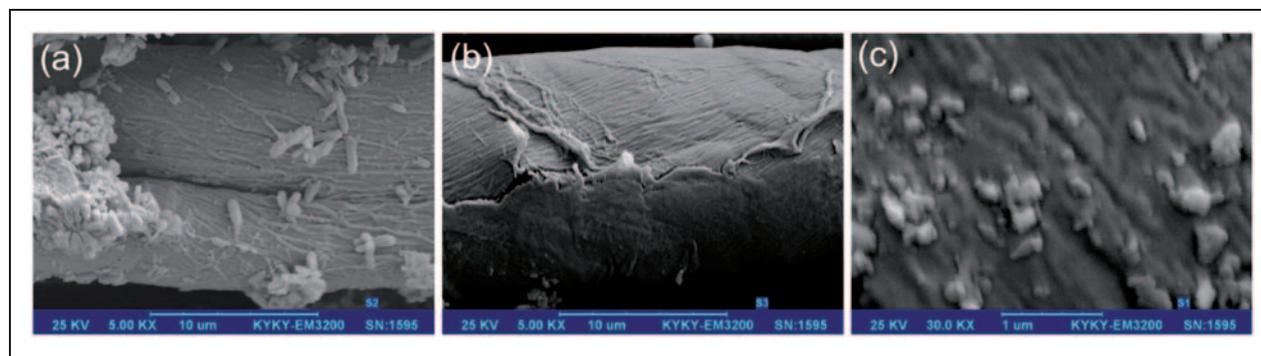
**Figure 5.** Scanning electron microscopy images of the ZnO-coated fabric after one (a) and five (b) cycles washing. Image (c) shows the higher-magnification of (b).
