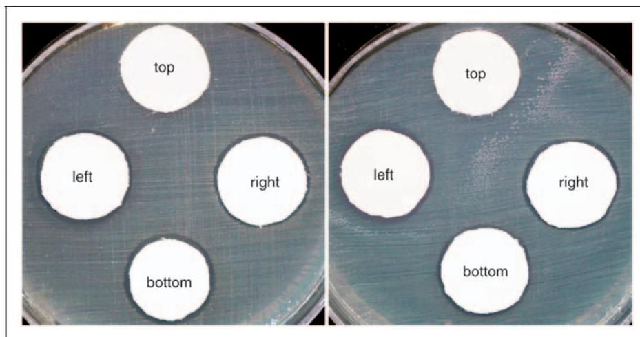
**Figure 3.** Antibacterial activities of the control fabric (top), the ZnO-coated fabric (right), the ZnO-coated fabric after one cycle of washing (bottom) and the ZnO-coated fabric after five cycles of washing (left), placed on the agar plate inoculated with *K. pneumonia*. The image on the right is for the same samples under ultraviolet radiation.
