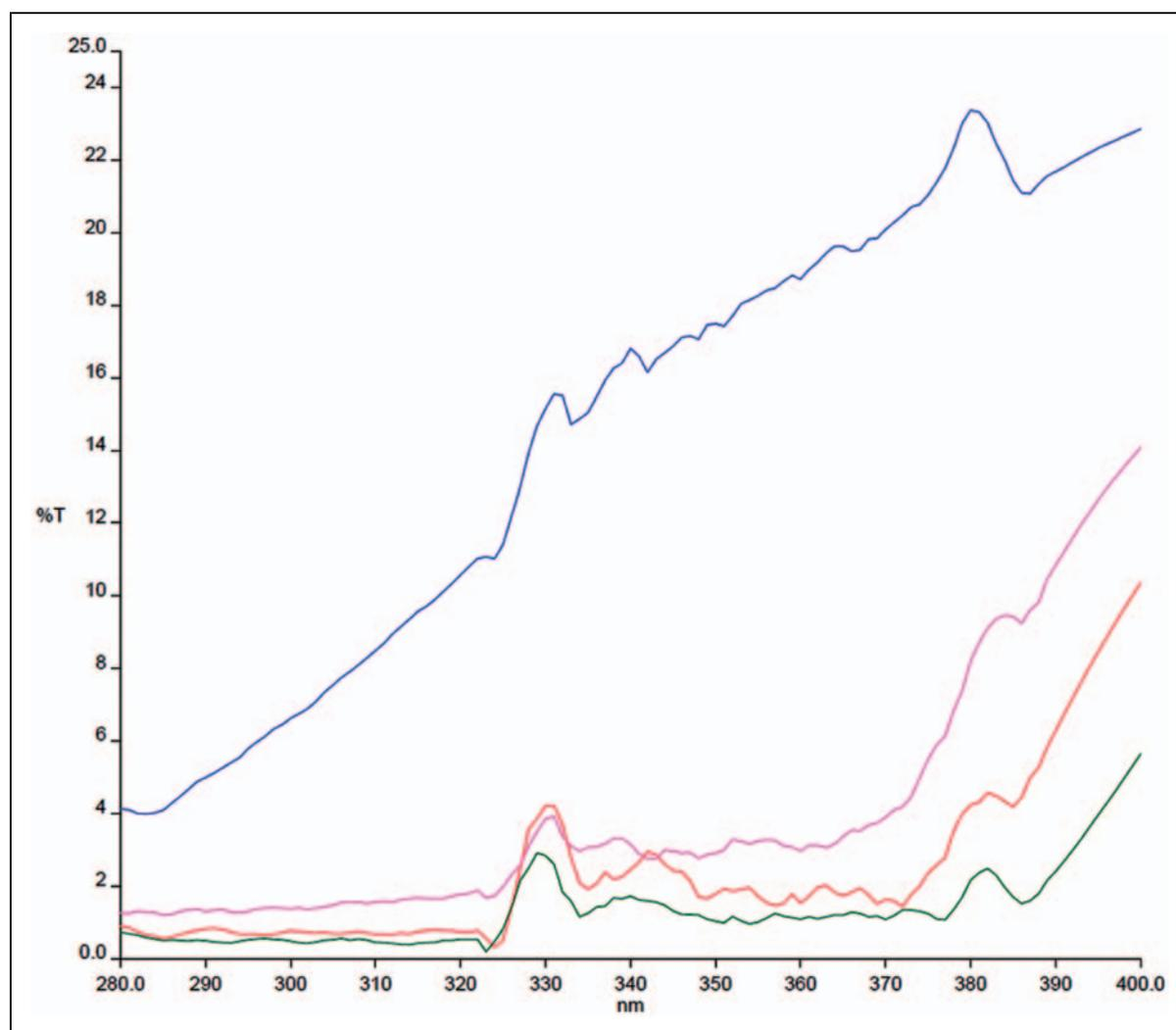
**Figure 6.** Ultraviolet-blocking spectra of the control fabric (blue line), the ZnO-coated fabric (red line), the ZnO-coated fabric after one cycle washing (green line) and the ZnO-coated fabric after five cycles washing (pink line). (Color online only).
