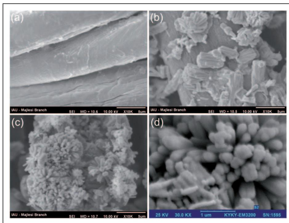
**Figure 1.** Scanning electron microscopy images of the control fabric (a) and the ZnO-coated fabric at different surface positions (b) and (c). The high-magnification image of the ZnO particle is shown in (d).
