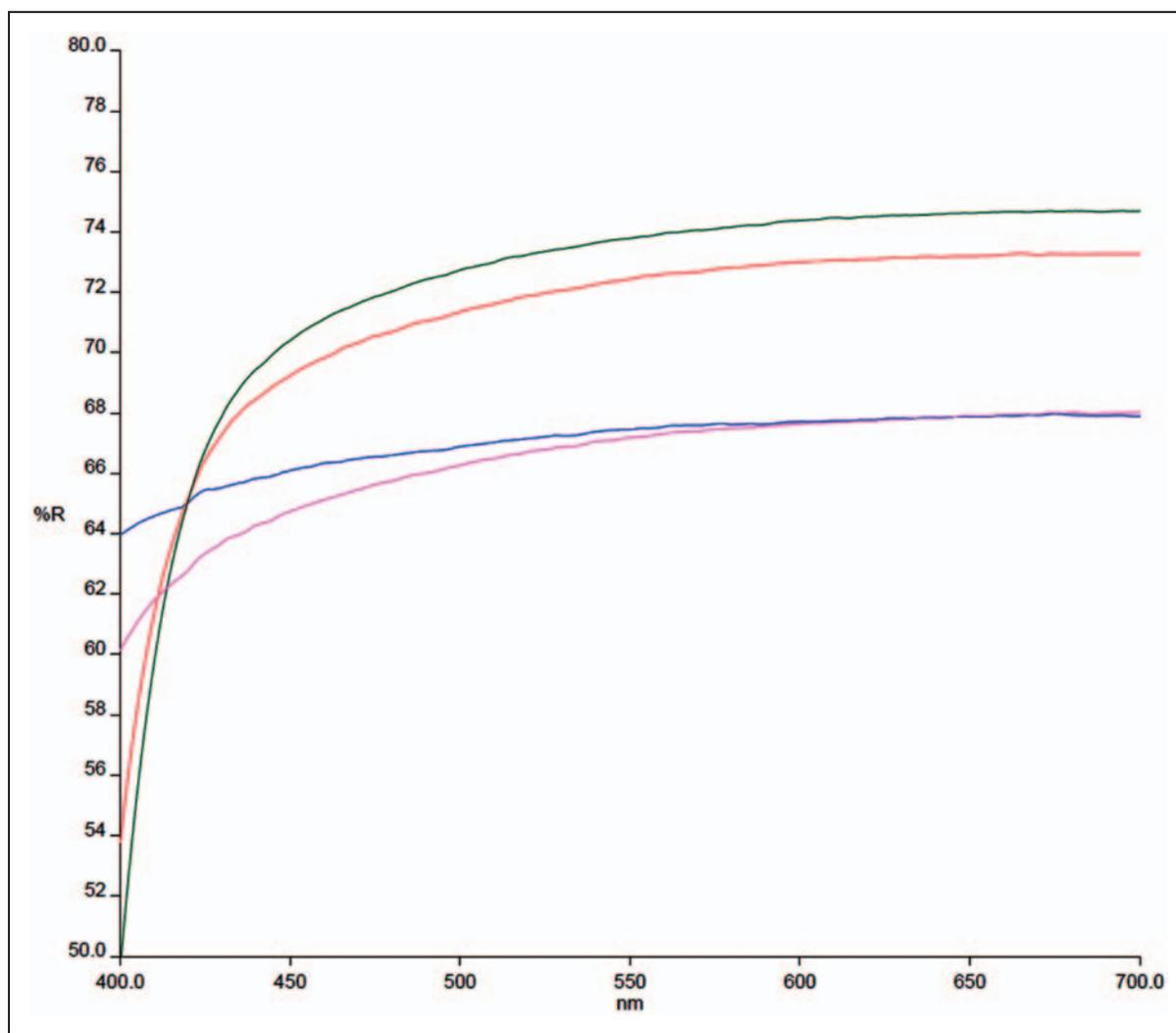
**Figure 7.** Visible spectra of the control fabric (blue line), the ZnO-coated fabric (red line), the ZnO-coated fabric after one cycle washing (green line) and the ZnO-coated fabric after five cycles washing (pink line). (Color online only).
