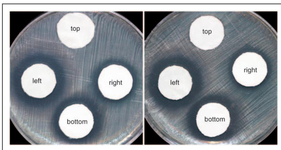
**Figure 4.** Antibacterial activities of the control fabric (top), the ZnO-coated fabric (right), the ZnO-coated fabric after one cycle of washing (bottom) and the ZnO-coated fabric after five cycles of washing (left), placed on the agar plate inoculated with *S. aureus*. The image on the right is for the same samples under UV radiation.
