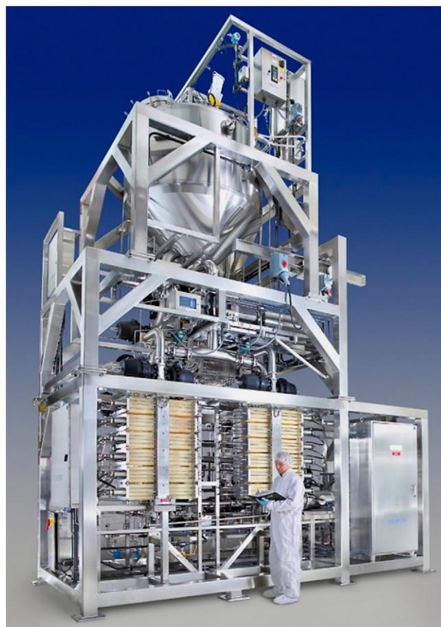
Fig. 18. High concentration UF system with 250 m<sup>2</sup> membrane area. New tank design with a retentate lift tube combined with close-coupling of all feed and retentate components in a vertical arrangement resulted in a minimum operating volume (including product in the recycle tank) while maintaining good mixing, minimal short-circuiting of retentate to feed, and no air entrainment. Photo used with permission of Genentech, Inc. and Millipore Corporation.
