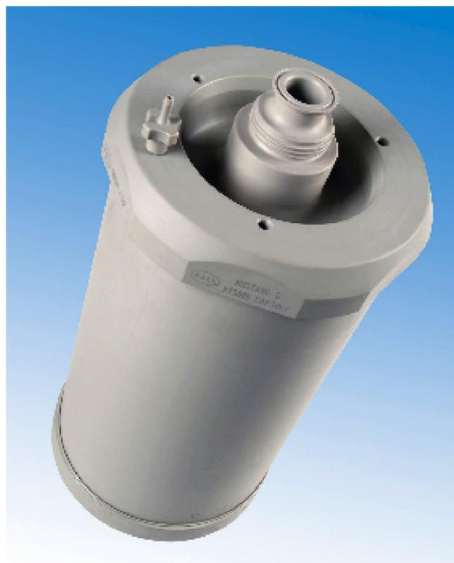
Fig. 12. Industrial scale membrane chromatography unit. Pall Mustang® 5L XT 5000 module with 16 layers of pleated 0.8 μm PES membrane with quaternary amine ligand. Photo used with permission of Pall Corporation.
