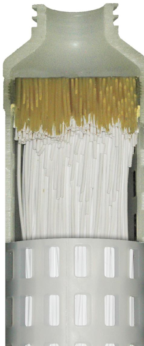
Fig. 7. Autoclavable hollow fiber cartridge with: (1) annealed polypropylene to eliminate polymer stress; (2) smaller diameter to reduce thermal expansion and contraction; (3) serrated bonding surface between polyurethane potting compound and polypropylene cartridge; (4) increased thickness of cartridge cage; and (5) inserted metal ring in cartridge outlet (not shown) to stabilize seal during heating and cooling. Photo used with permission of Genentech, Inc.
