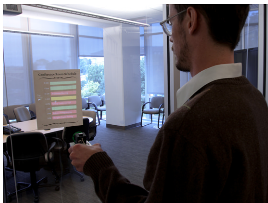
Figure 10. The Schedule Viewer application enables a static sign to be augmented with projected information from a conference room schedule.
