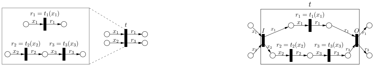
Fig. 2. Hierarchical workflows: a composite transition representing a subworkflow (left) and a semantically equivalent HLPN without composite transitions (right).
