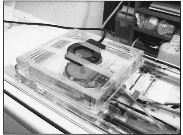
Fig. 1. Plexiglas tissue sample holder positioned above the HIFU transducer. The liver specimen is positioned in a water bath and completely covered by degassed water. A circular RF coil is placed on top of the tissue sample and taped to the holder to minimize motion.
