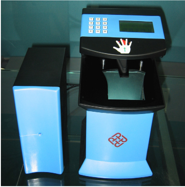
Fig. 5. A CCD-based palmprint scanner.
