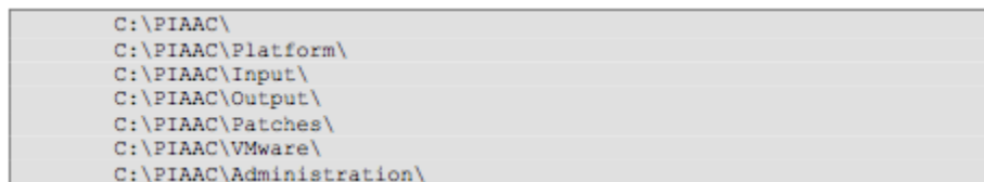
Figure 7.9: Structure of the shared folder between the PIAAC VM and the laptop host system for file exchange
