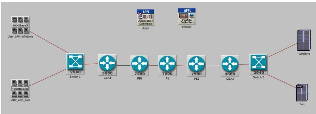
Figure 4. OPNET Network Setup
