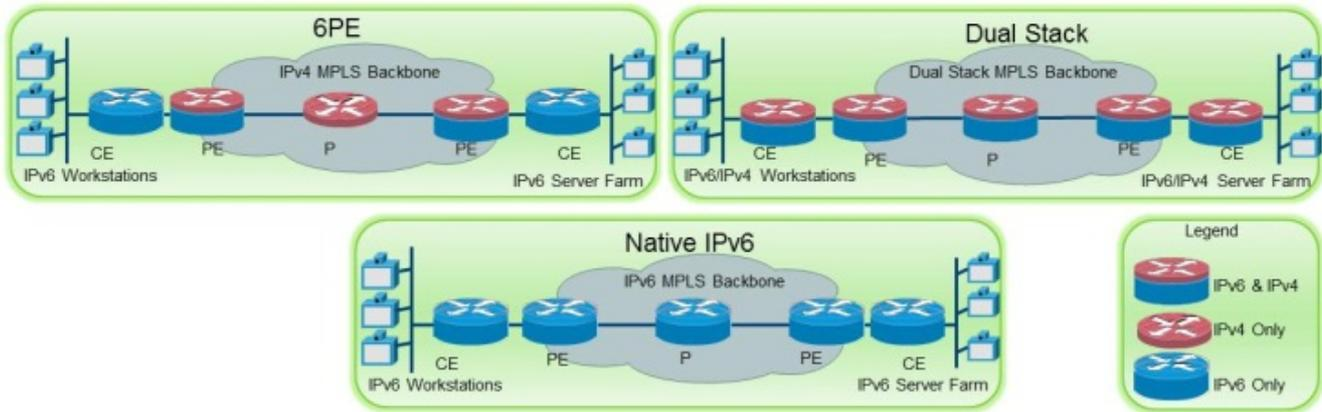
Figure 3. 6PE, Dual Stack, and Native IPv6 Transition Mechanisms
