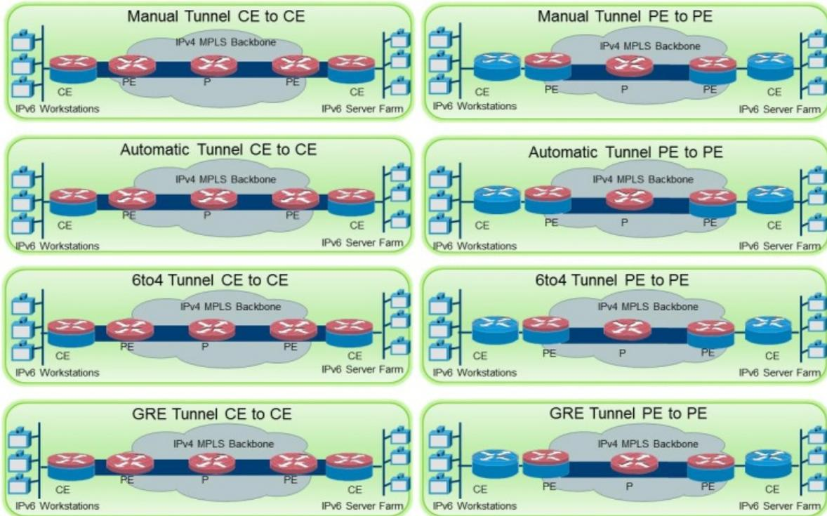
Figure 2. CE-to-CE and PE-to-PE IPv6 Tunneling Mechanisms
