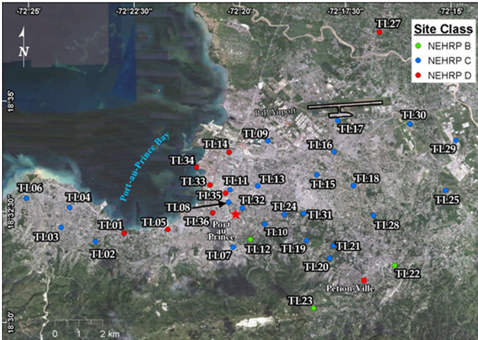
Figure 3. Locations and names of sites in Port-au-Prince, Haiti where multichannel analysis of surface waves (MASW) testing was performed to obtain shear wave velocity profiles (image courtesy of Google Earth, ©2009 Google).
