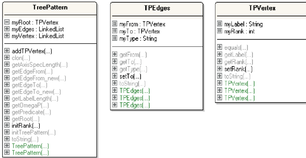
Figure 8.6: UML-diagram for the tree pattern and its components
