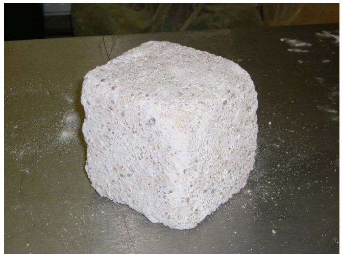
Fig. 6. Typical 100% portland cement mortar sample after final stage of immersion
