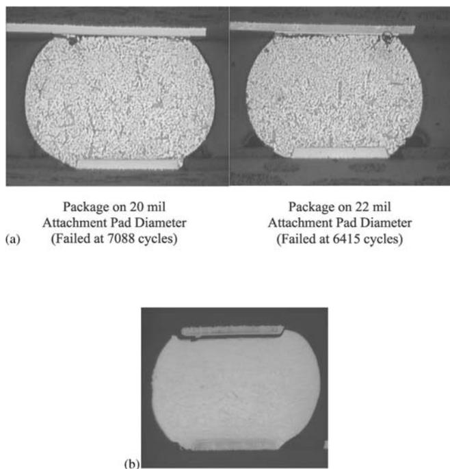
**Fig. 2. a** Examples of fatigue failure for different PCB pad sizes **b** Example of a non-fatigue failure
