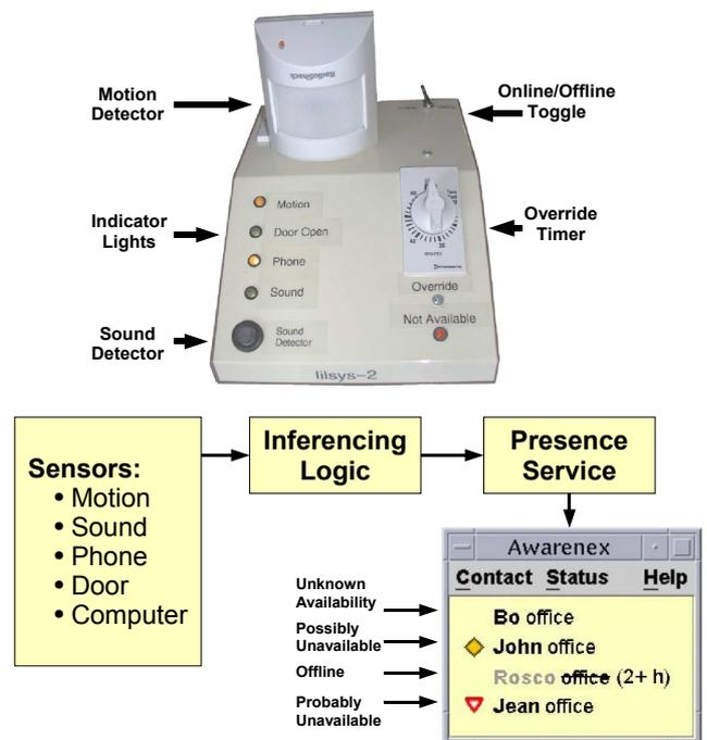
**Figure 22.10.** Above: LILSYS’s sensor and data acquisition module; below: the system’s data flow and a screen shot of the user interface. (Adapted from Figures 1 and 2 of: “Lil-sys: Sensing unavailability,” by J. Begole, N. E., Matsakis, & J. C. Tang, 2004, In J. Herbsleb & G. Olson (Eds.), *Proceedings of the 2004 Conference on Computer-Supported Cooperative Work*, pp. 511–514, New York: ACM. Copyright 2004 by ACM. Adapted with permission.)
