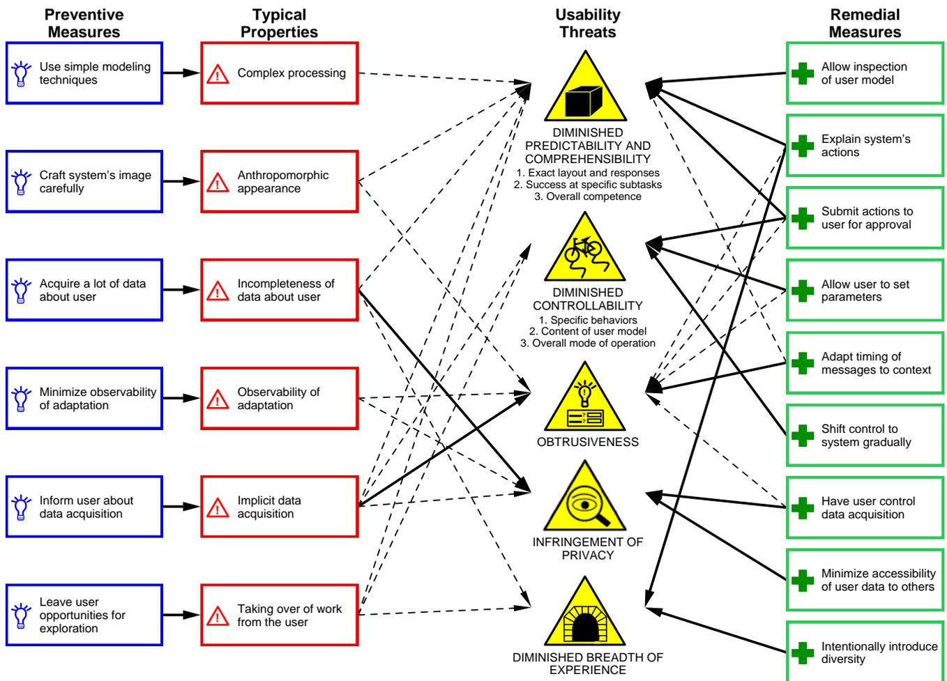
**Figure 22.23.** Overview of usability challenges for user-adaptive systems and of ways of dealing with them. (Dashed arrows denote threats and solid arrows mitigation of threats, respectively; further explanation is given in the text.)
