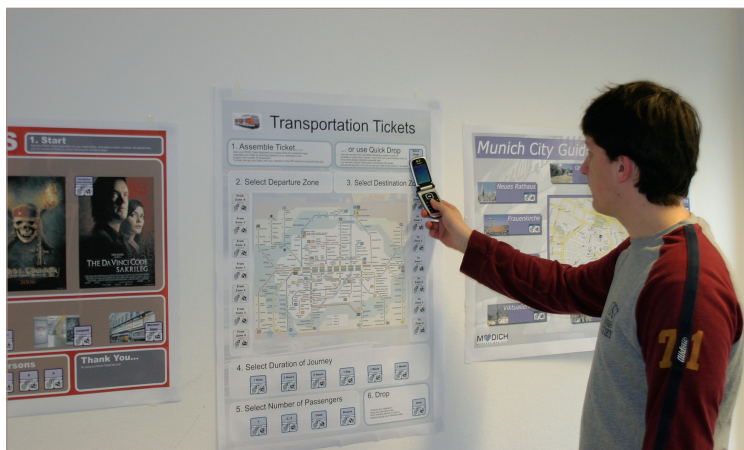
Figure 1. Physical mobile interaction (PMI) with multiple tags and objects. Tagged objects can serve as physical user interfaces that facilitate interaction with associated information and services. (Research prototypes include material from www.actuacine.net and www.mvg-mobil.de .)
