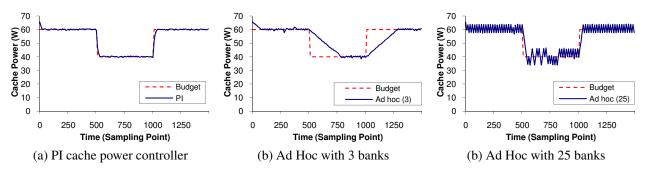
Figure 2. Typical runs of the PI cache power controller and a baseline under a power budget reduction.
