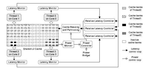
Figure 1. Two-tier L2 cache control architecture for power capping and fair/differentiated sharing.
