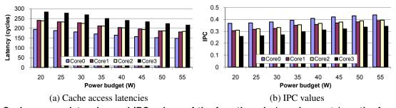
Figure 4. Cache access latencies and IPC values of the four threads (running *crafty*) on the four cores of the CMP. When power budget varies from 20W to 55W, all the threads have reduced cache latencies and increased IPCs, while the desired latency differentiations and fairness are maintained.
