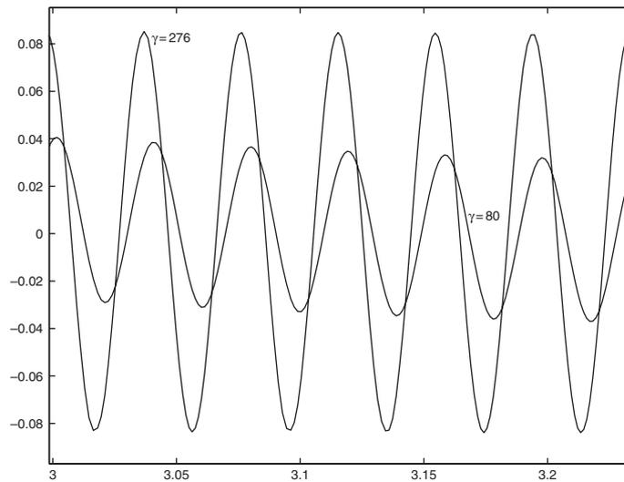
Figure 3. The error  $x_1(t) - \hat{x}_1(t)$  versus time for different observer gains.
