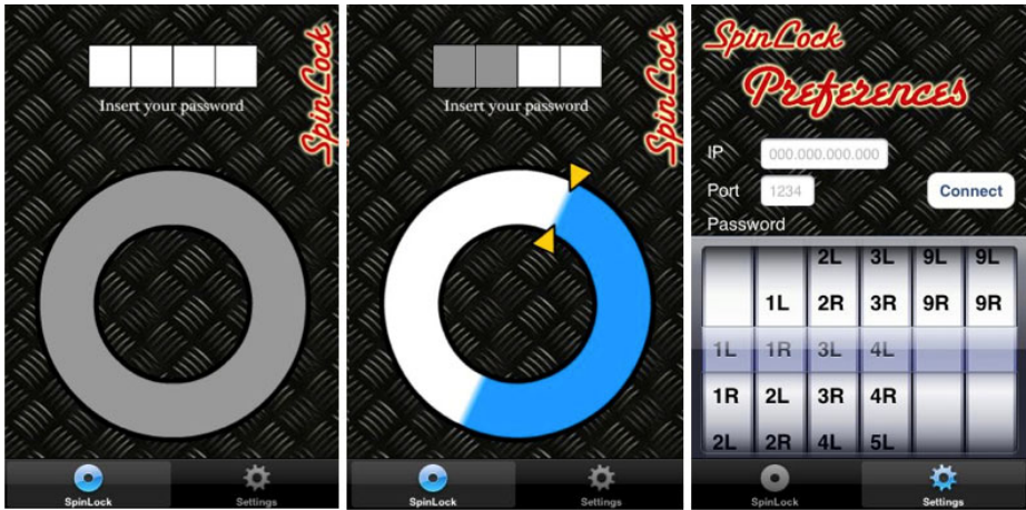
Fig. 2. The Spinlock graphical user interface: whilst idle (left), during the user interaction with two PIN items entered (center) and the settings screen showing user password (right)
