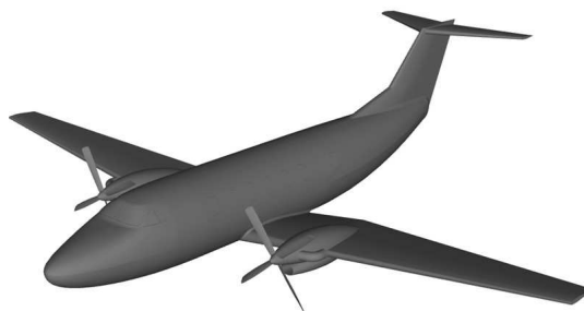
Figure 4.7: Perspective view of a Beechcraft produced from a three-dimensional CAD model [210].
