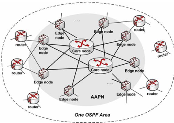
Fig. 1: Agile All-Photonic Network overlaid star topology.
