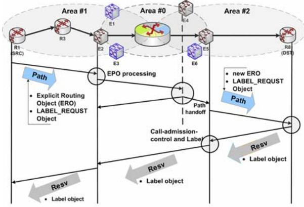
Fig. 5: Inter-area LSP signaling process
