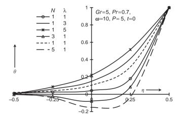
Figure 9. Temperature distribution for N and  $\lambda$  at t=0
