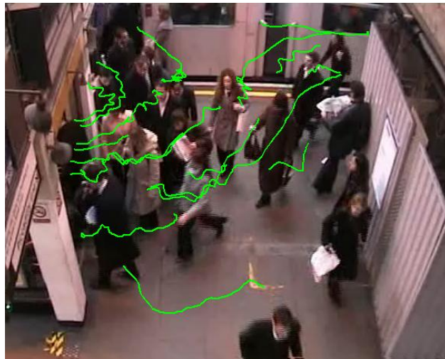
Fig. 3. Some of the longest point tracks extracted from a crowd scene video. The point tracks are overlaid on one of the frames from the video sequence.
