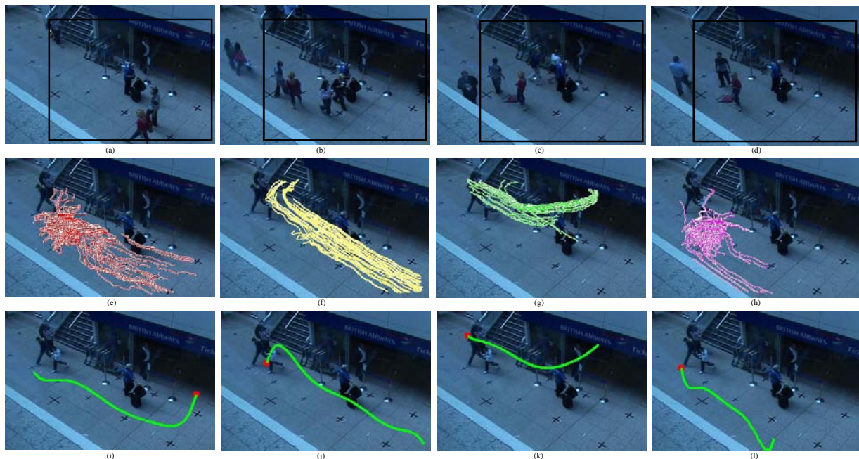
Fig. 11. (a)-(d) Example frames from the airport sequence . The rectangular box overlaid on the frames denotes the region where analysis was performed. (e)-(h) Trajectories belonging to the four different clusters identified by the algorithm. (i)-(l) The cluster centers generated by the algorithm correspond to the dominant motions in the video sequence: (i) crossing from right to left, (j) crossing from left to right, (k) entering the ticketing office from the left, (l) entering from the right and loitering. (This figure is best viewed in color.)
