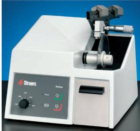
Figure 3.5 Struers Minitom used for specimen cutting.
