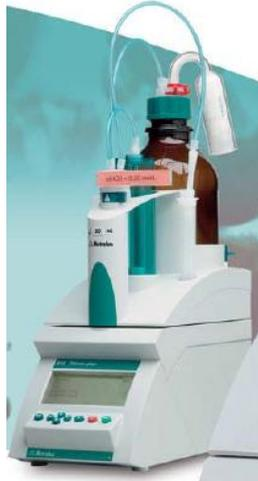
Figure 3.8 Titration 877 automatic titration machine for chloride content determination.
