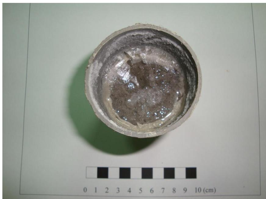
Figure 4.18 Salt crystal formations on concrete surface.
