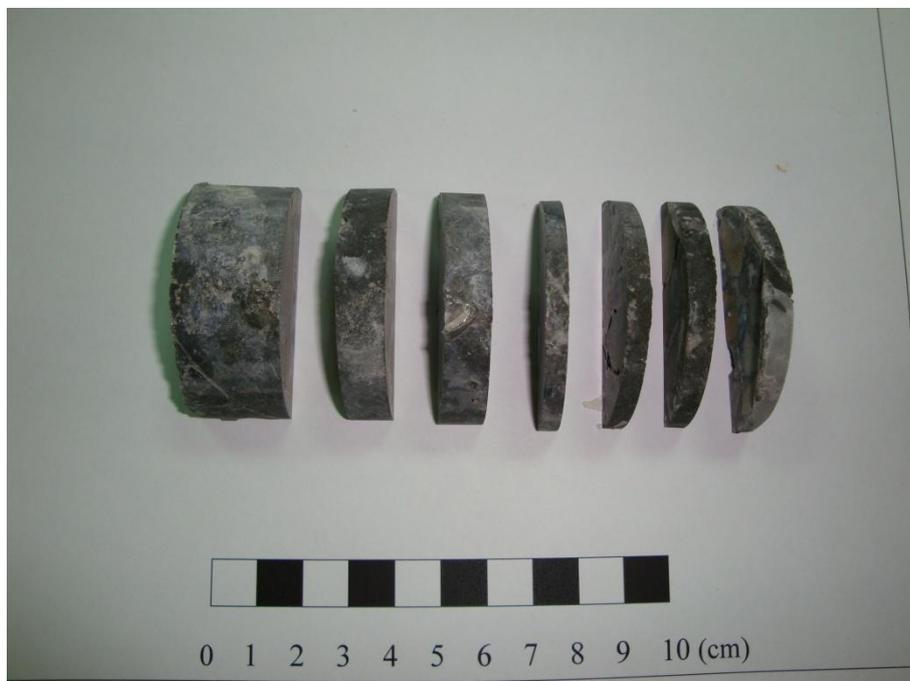
Figure 3.6 Sliced specimen for the profiling of chloride concentration at various depths
