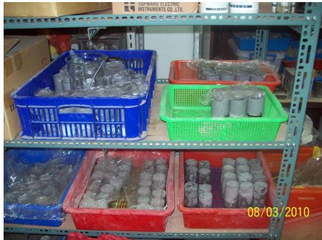
Figure 3.4 Specimen storage condition during salt ponding test
