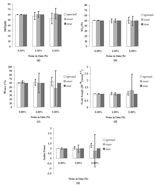
Fig. 1. Recovered mean values with standard deviation error bars are shown for (a) hemoglobin, (b) oxygen saturation  $(SO_2)$ , (c) water (in percent), (d) scatter amplitude, and (e) scatter power. These were estimated from the interior of a homogeneous field reconstructed with different levels of noise in the original data. Values for the new spectrally constrained reconstruction are shown alongside results from the conventional approach.
