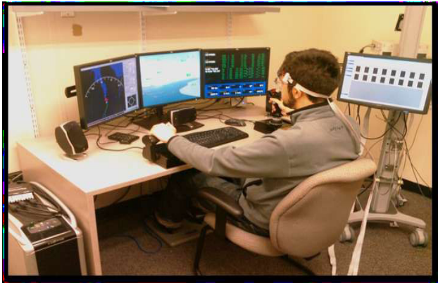
Fig. 4. Subject operating the Predator UAV simulator with fNIR sensor attached and data acquisition apparatus on far right
