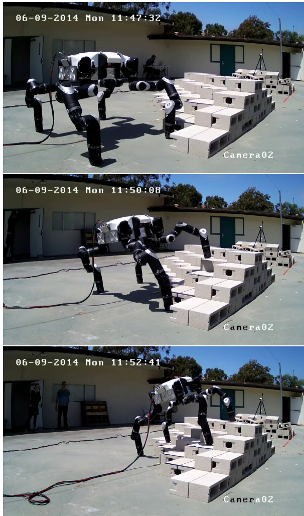
Figure 10: We used our approach with real robot hardware in an outdoor environment. Results were similar to simulations, but we were substantially limited by issues related to perception and localization. The system was able to proceed as far as shown before the robot’s pose estimate error became too large for it to plan successfully. Before this occurred, it planned and executed 19 steps fully autonomously.
