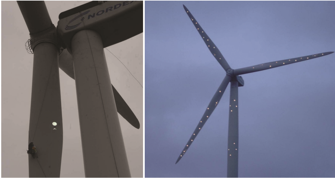
Figure 3.1 a-b. Placement of markers and their final layout on the turbine 29 .
