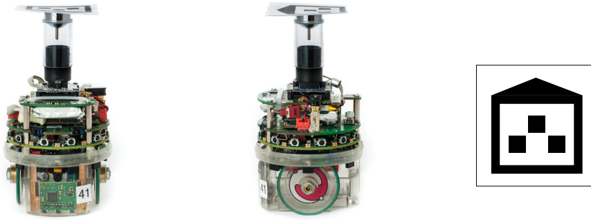
Fig. 1: Front and side view of an e-puck robot and a tag used to localize the robot via a ceiling-mounted camera
