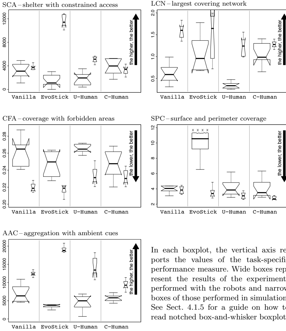
Fig. 4: Study A—notched box-and-whisker boxplots of the results obtained by Vanilla , EvoStick , U-Human , and C-Human on the five tasks
