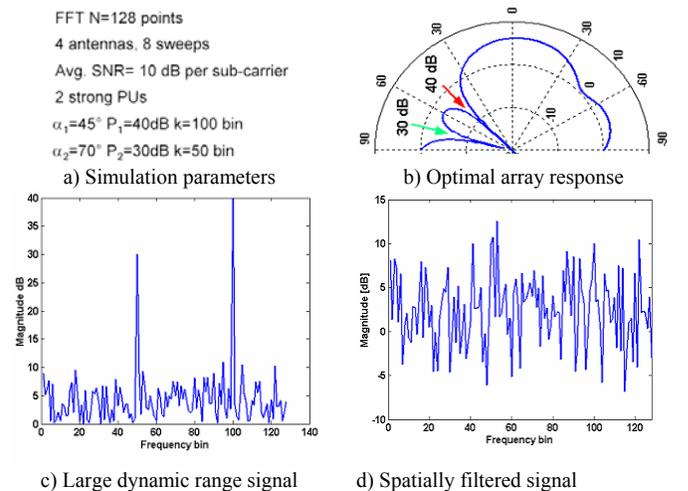
Figure 4. An example of dynamic range reduction using antenna arrays
