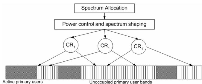
Figure 5. Cognitive radio wideband spectrum access
