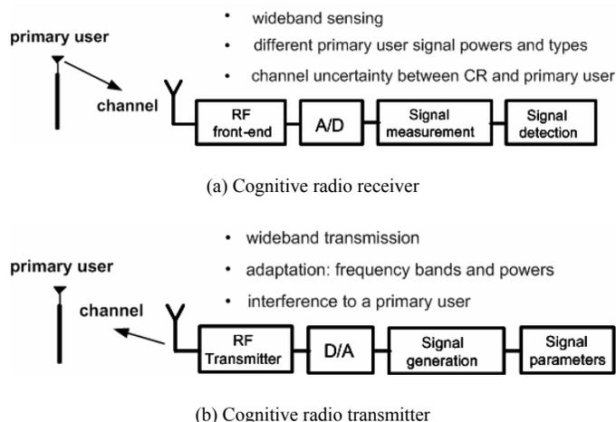
Figure 1. System issues in unique cognitive radio physical layer functions
