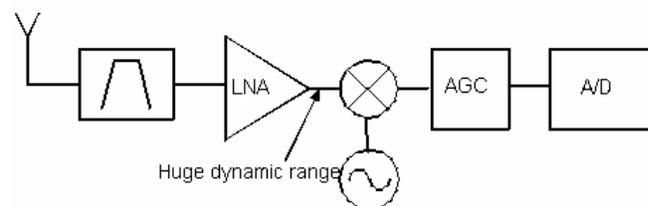
Figure 2. Wideband cognitive radio RF front-end
