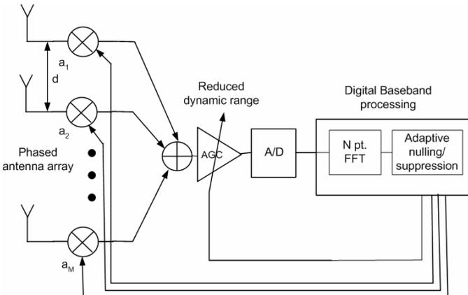
Figure 3. Wideband RF front-end with antenna array for spatial filtering
