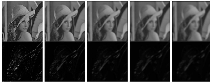
Fig. 12. Gaussian scale space images of Lena (top row) and of the Gabor filtered version of Lena (bottom row). While the gray-value image degrades gracefully, revealing structures at different scales, the sparse edge image fades away.
