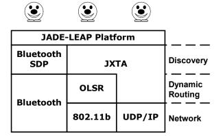
Figure 1: The "Big" Picture. The modified JADE-LEAP platform will utilise existing discovery and routing technologies.
