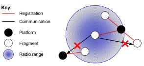
Figure 4: Wireless networks are not fully connected. An agent discovered through a directory may not be contactable due to the limitations of the wireless technology and the routing protocols in use.
