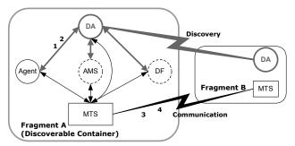
Figure 5: Overview of the modifications to JADE-LEAP. Grey indicates new discovery-related communications or components. Dotted lines indicate an optional component.
