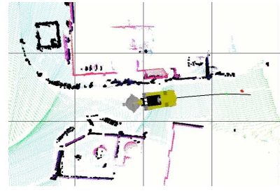
Fig. 10. A 2D visualisation of an 'obstacle detected' event in the 3D obstacle detection system. The HMC is the yellow object with the grey crucible attached behind it (left). The HMC's path is shown as the black line projected to the right. Environment features are shown in black and pink with the groundplane as the green dots. Along the vehicle's projected path is a red object (traffic cone). Since this object occurs within the width of the vehicle along its path, it is considered an obstacle.
