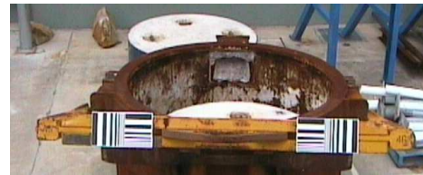
Fig. 7. The visual fiducials used to uniquely identify the crucible in the environment.
