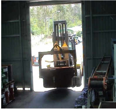
Fig. 5. Entry to the storage shed where the crucible gets dropped off. Note the clearance between the vehicle and the doorway sides is less than 20cm. The vehicle successfully traverses through the doorway using waypoints which demonstrates the accuracy and repeatability of the localisation, navigation and control systems.
