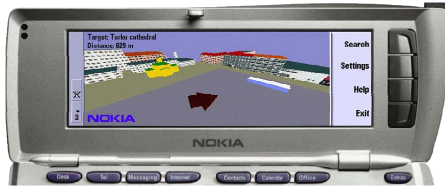
Figure 1. Project Tellmaris employed location sensing to display three-dimensional models of the user locality overlaid with tourist information. This figure shows the client application interface which allows users to navigate the model and discover landmarks and services while visiting the site.
