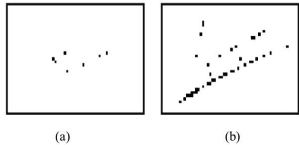
Figure 7. (a) Common pixels of two reduced sample signatures before registration (b) Common pixels of two reduced sample signatures after registration.
