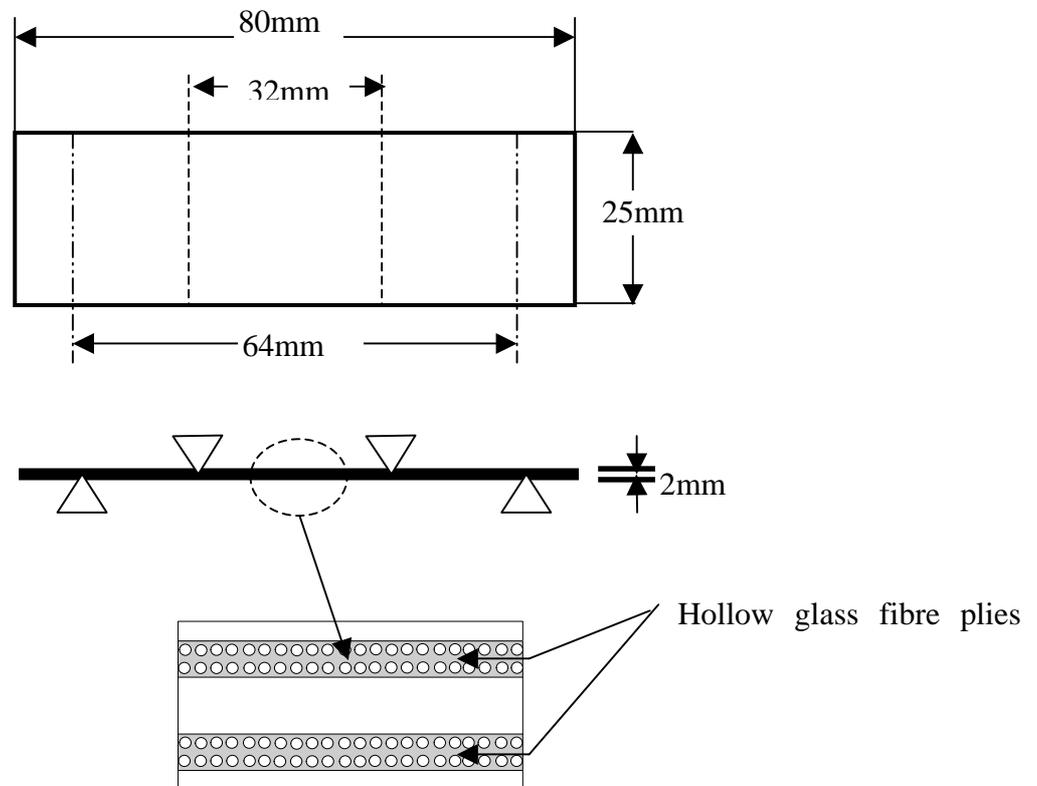
**Figure 2.** Lay-up configuration and dimensions for 4-point bend flexural testing.
