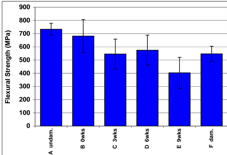
**Figure 4.** Results of flexural testing for damaged, undamaged and self-repaired specimens after various storage periods (bars denote standard deviation).
