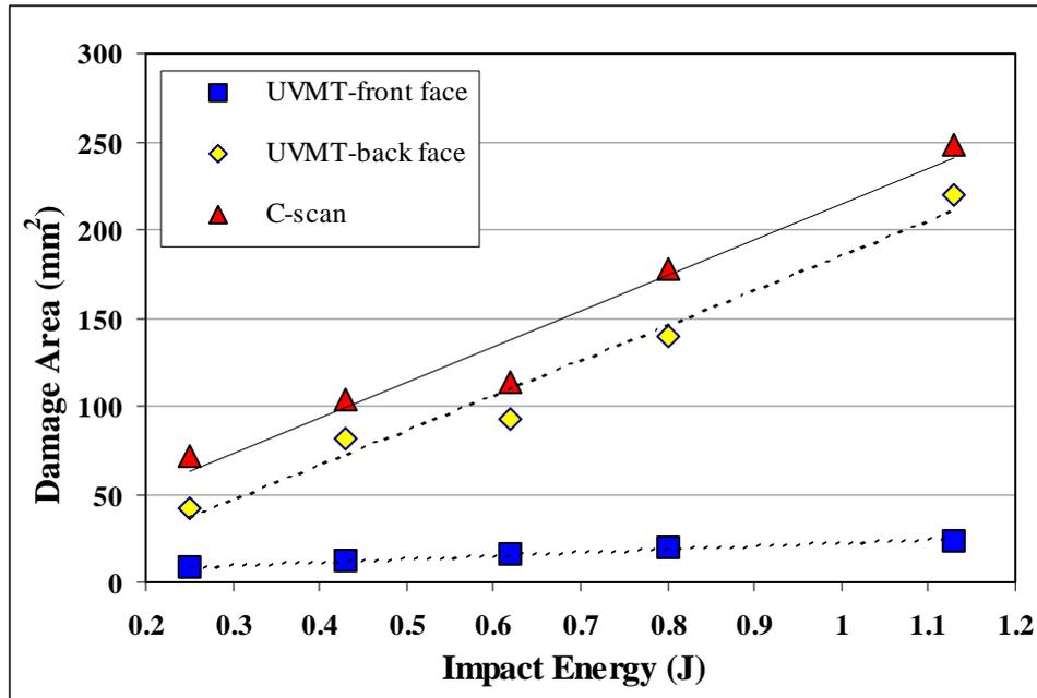
**Figure 6.** Correlation of damaged area measured by UVMT (from front and back faces) and ultrasonic C-scan.
