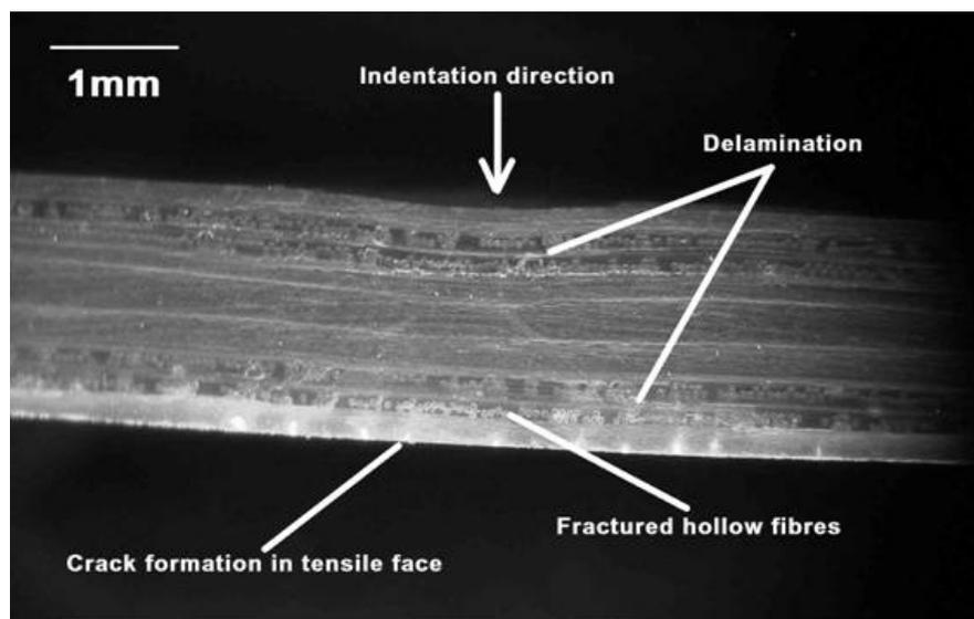
**Figure 3.** Optical micrograph of cross-section through impact damaged hybrid solid glass/hollow glass/epoxy laminate.
