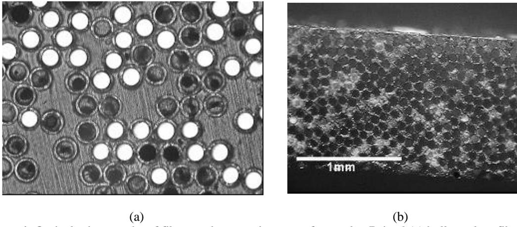
**Figure 1.** Optical micrographs of fibres and composites manufactured at Bristol (a) hollow glass fibres of 60µm external diameter with a hollowness of 50% and, (b) the same fibres within a Hexcel 913 epoxy matrix
