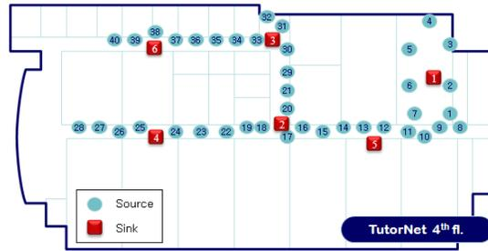
Fig. 20. Layout of source and sink nodes in TutorNet.
