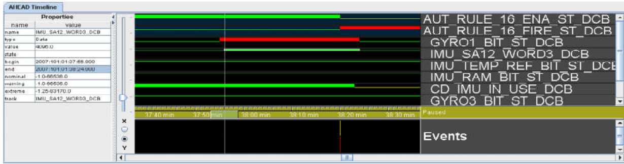
Figure 11. Temporal view of autonomous activity in a STEREO spacecraft. A temporal view shows autonomous activities, goal accomplishment, environmental events and system responses over time, at selected levels of abstraction.
