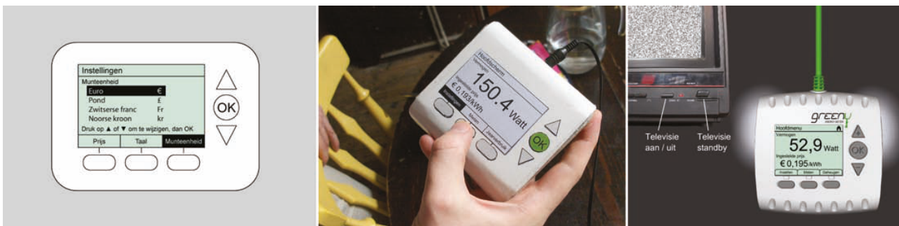
Figure 4: Wever, Kuijk & Boks illustrate on-screen (left), physical simulations (middle) of the product during user evaluations (middle and right), demonstrating a process incorporating iterative delivery and prototyping with observational research.
