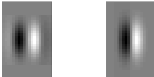
Fig. 5.5: Left: Weighting function resulting from successive convolution of filter masks used to compute the complex cell responses. Right: Fit of a first order Gaussian derivative mask with standard deviations \sigma_{x,\text{fit}} = 1.96 and \sigma_{y,\text{fit}} = 4.45 .
