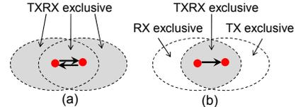
Fig. 1: Spatial reuse in (a) full-duplex and (b) half-duplex networks. Dotted lines denote interference range. RX (TX) exclusive region can be reused by other TX (RX). But TXRX exclusive region cannot be reused by others.
