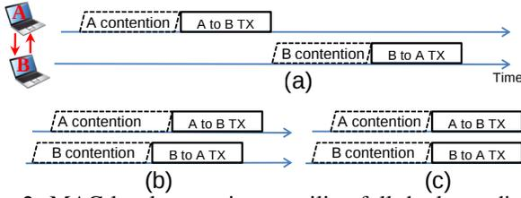
Fig. 2: MAC-level strategies to utilize full-duplex radios: (a) Half-duplex access; (b) Opportunistic full-duplex access; (c) Semi-synchronous access.
