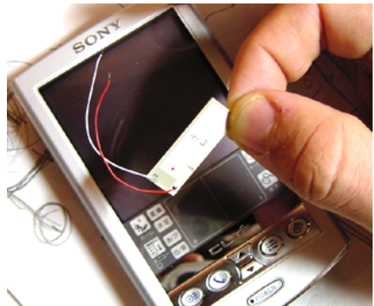
Figure 1: TouchEngine™ actuator – a new vibrotactile actuator for designing tactile interfaces for small handheld computing devices; it is only 0.5 mm thick
