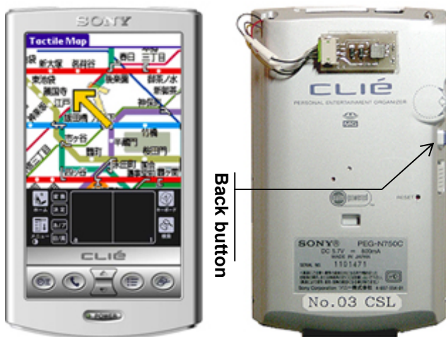
Figure 8 Tilting interfaces: 2D browsing of a Tokyo subway map. Tilt sensor board is attached on the back.
